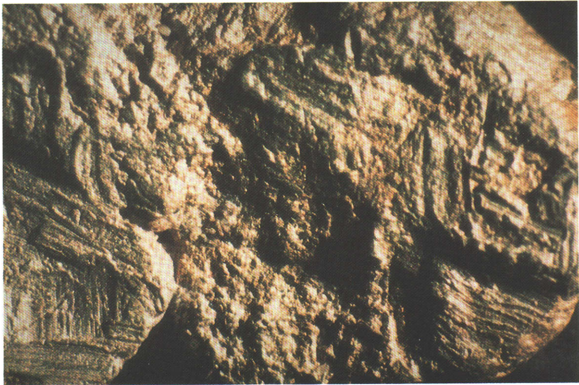
Figure 67 - Striations on a flat gold specimen from Klaza River. Field of view 5 mm.
