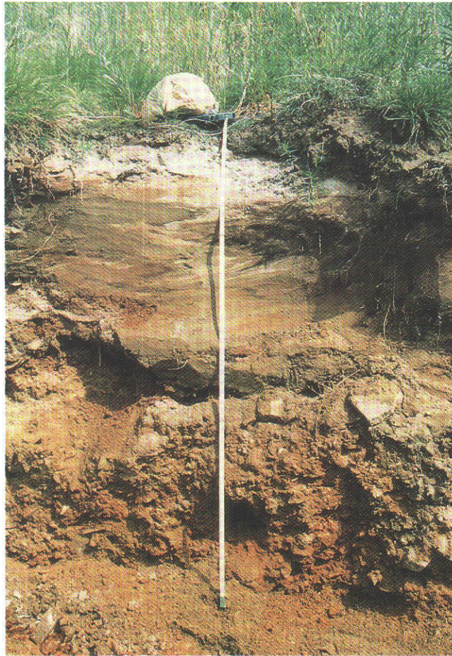
Figure 16 - Stratified silt and clay of Facies 4 overlies disorganized pebble-cobble gravel of Facies 9 at Eva Creek section EVA 1-1, and is in turn overlain by White River Ash. Traces of an older tephra are mixed with the silt and clay.
