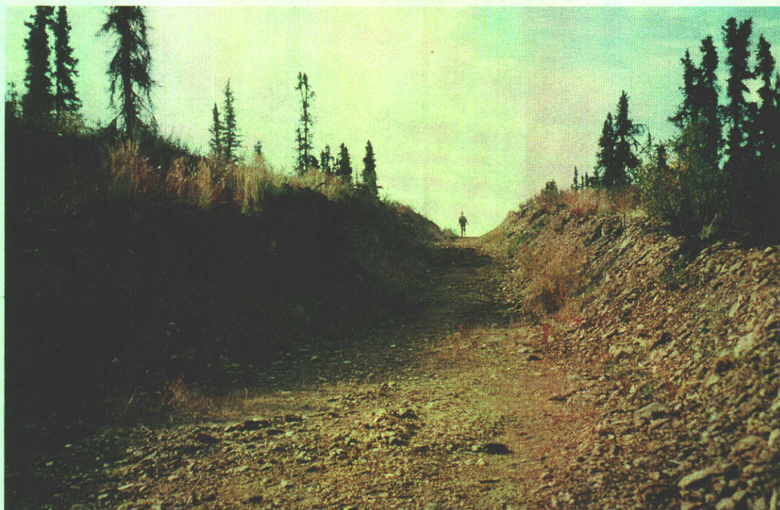
Plate 2-8 Trench 88TR20, sites 88TR2a, 88TR2b and 88TR2c. Vegetation patches visible on the wall are slumping from the surface. Pioneer vegetation is concentrated at the toe of the colluviated material.
