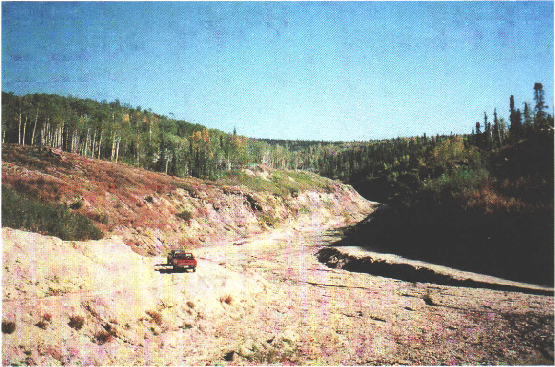
Plate 5-3 Overview of Oro Grande Operation. Cuts (on the right) and overburden/tailing piles (left) are younger upcreek.
