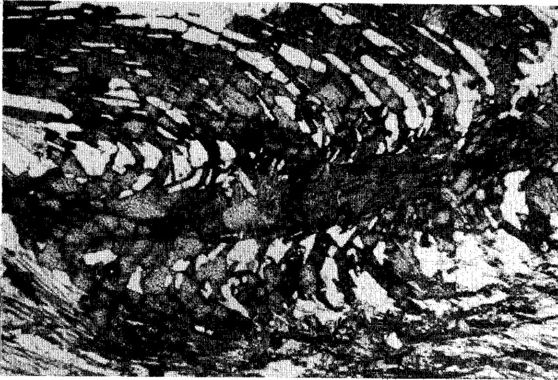
Figure 18a: Garnet porphyroblast superimposed over D2 fold of S1 outlined by elongate quartz grains. Growth of garnet therefore post-dates D2 folding.
