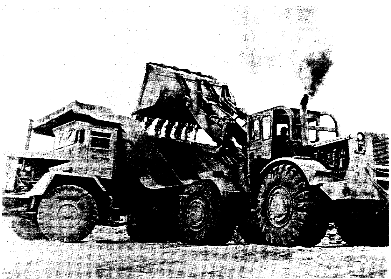
Photo 5: Open pit mining: side view showing 35 ton Euclid truck being loaded.
