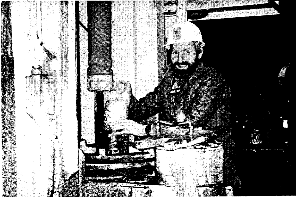
PHOTO 2 Dropping (Air Mailing) the Radiotracer Test Core
