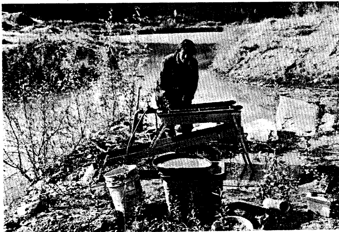
PHOTO 4 Concentrating Drill Samples with a Long Tom
