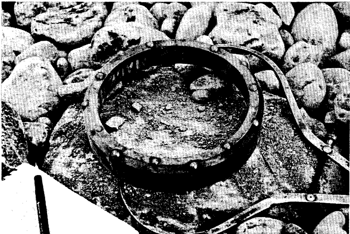
PHOTO 12 Barber DR Casing Shoe Studded with Carbides
