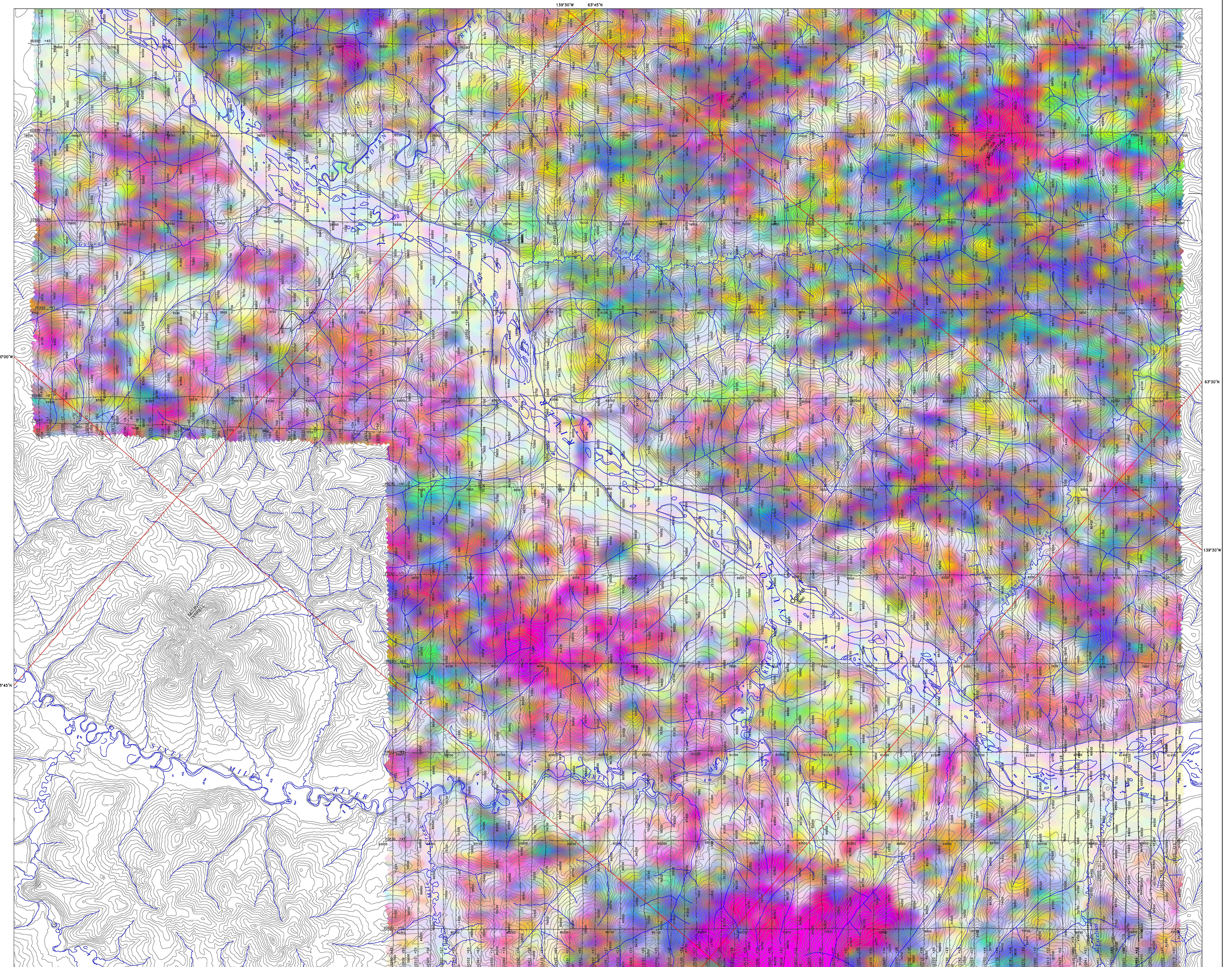
This map was compiled from data acquired during an airborne geophysical survey. Gamma-ray spectrometer, magnetometer and VLF data were collected by Fugro utilizing an AgustaWestland AS350B2 helicopter (registration C-FZTA). The survey operations were carried out from July 29, 2000 to September 1, 2000.
