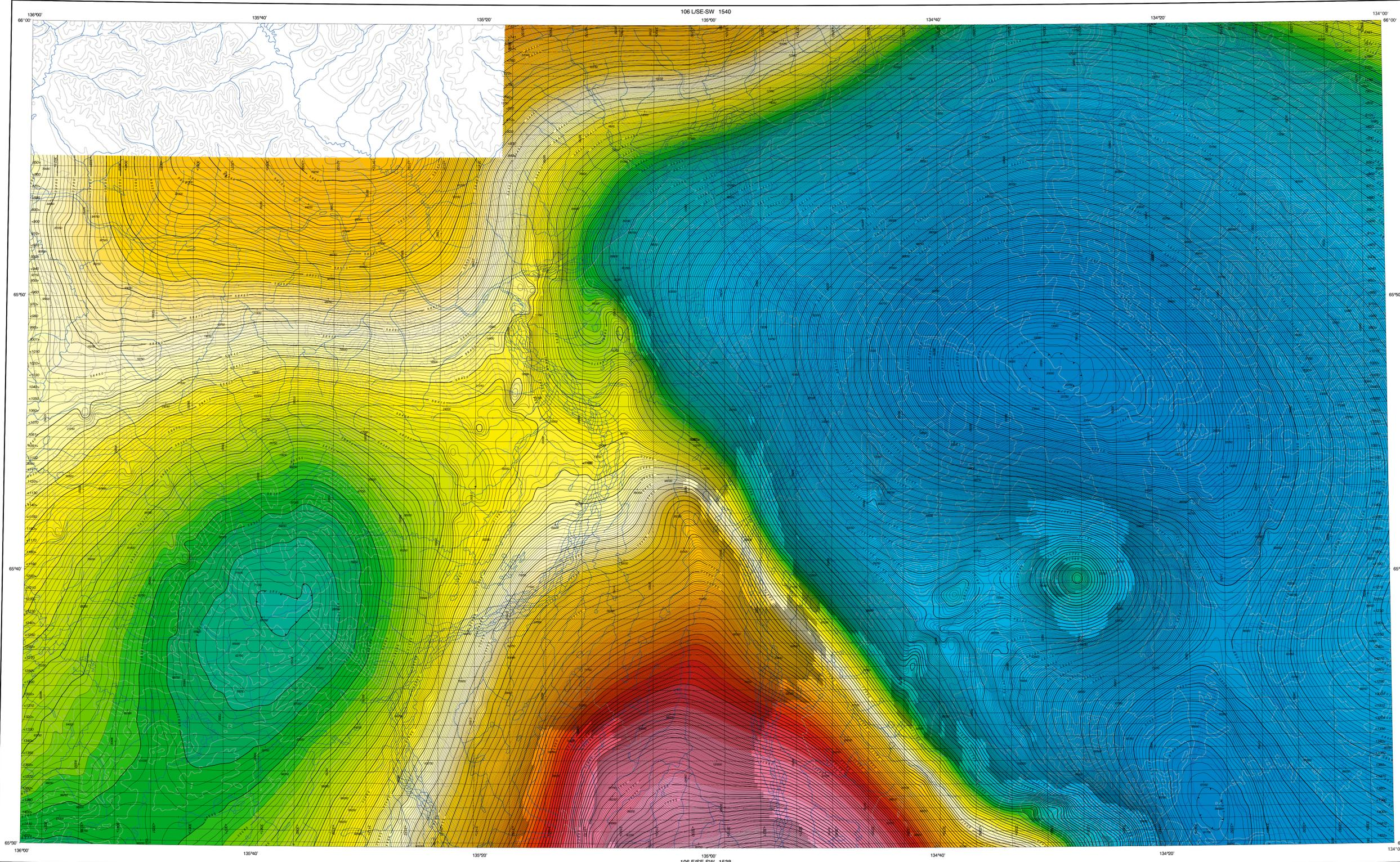
This map was compiled from data obtained as a result of an aeromagnetic survey carried out by Fugro Airborne Surveys using a Cessna Caravan ( registration CF-ZLX) aircraft. A 0.025 nT sensitivity split-beam cesium vapour magnetometer was mounted in the tail boom of the survey aircraft.
