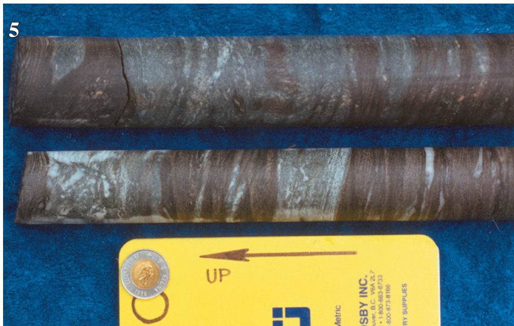
Photo 5. Core samples of the Transition Zone metasedimentary rocks (unit 2). Top core is from Hole 97-97 (255.6 m); the lower core is from Hole 97-115 (617.9 m). Both samples are of intercalated brown biotite-rich schist (after fine-grained felsic metasandstones) and green chlorite-actinolite schist (after fine-grained mafic metavolcaniclastic rocks). Pale carbonate is contained in the mafic volcaniclastic layers in the lower core. Both cores contain syndepositional features. The upper core displays lensey discontinuous green volcaniclastic beds, and displays possible scouring of an upper contact of green volcaniclastic by brown metasandstone just below the crack in the upper section of the core sample. Alternating finer grained dark brown versus lighter relatively coarser grained bands make-up the metasandstones of the lower core and these may be the product of small turbidites. The bedding displays angular contact relationships, which are possibly the product of cross-bedding.
