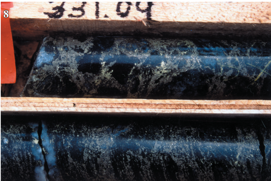
Photo 8. Close-up photo of fragmental-textured fine-grained magnetite cemented by pyrite, pyrrhotite, chalcopyrite and quartz. A quartz veinlet with chalcopyrite patches cuts the lower core at left. The core is from the West Kona Zone cored in Hole 97-95 (331 m).
