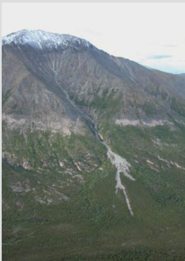
Figure XIII. Oblique photograph of debris-flow catchment and fan. A debris flow in the early 1990s came within 60 m of a proposed pipeline easement situated in the valley bottom (foreground).
