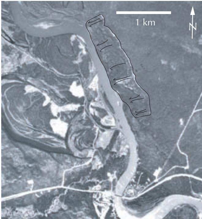
Figure 31. Aerial photograph of large rock slumps (outlined in black) within Pleistocene basalt and till adjacent to the Alaska Highway's crossing of the Liard River (National Air Photo Library number A27829-56, Natural Resources Canada).
