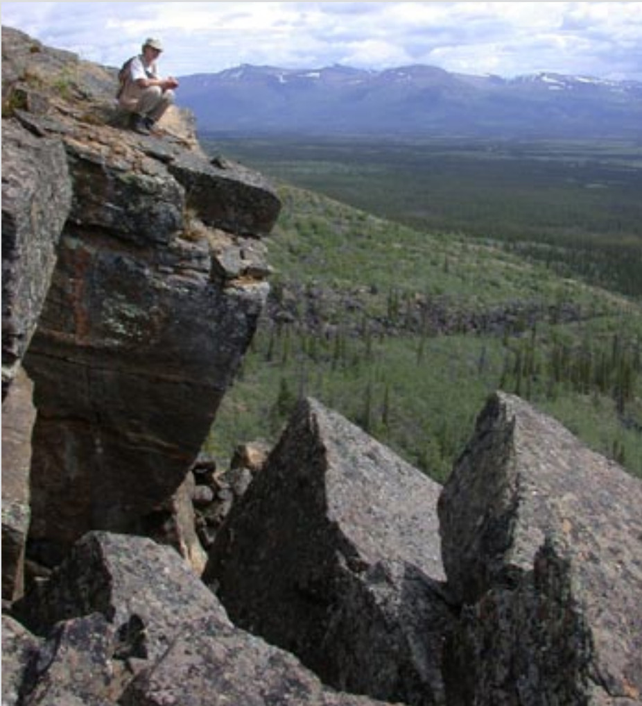
Figure X. Active toppling on western flank of Aishihik rock slide. The toppling movement has disturbed roots of live vegetation in adjacent hillslope.
