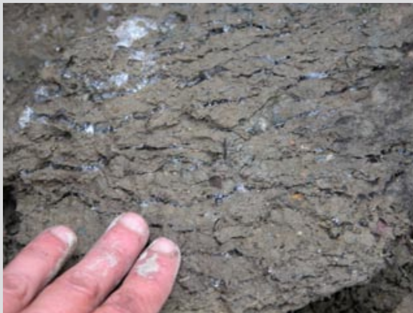
Figure XVI. Soil from beneath the permafrost table from unburned forest site displaying stratified visible ice. Thawing of ice-rich soil causes a significant loss of soil strength.
