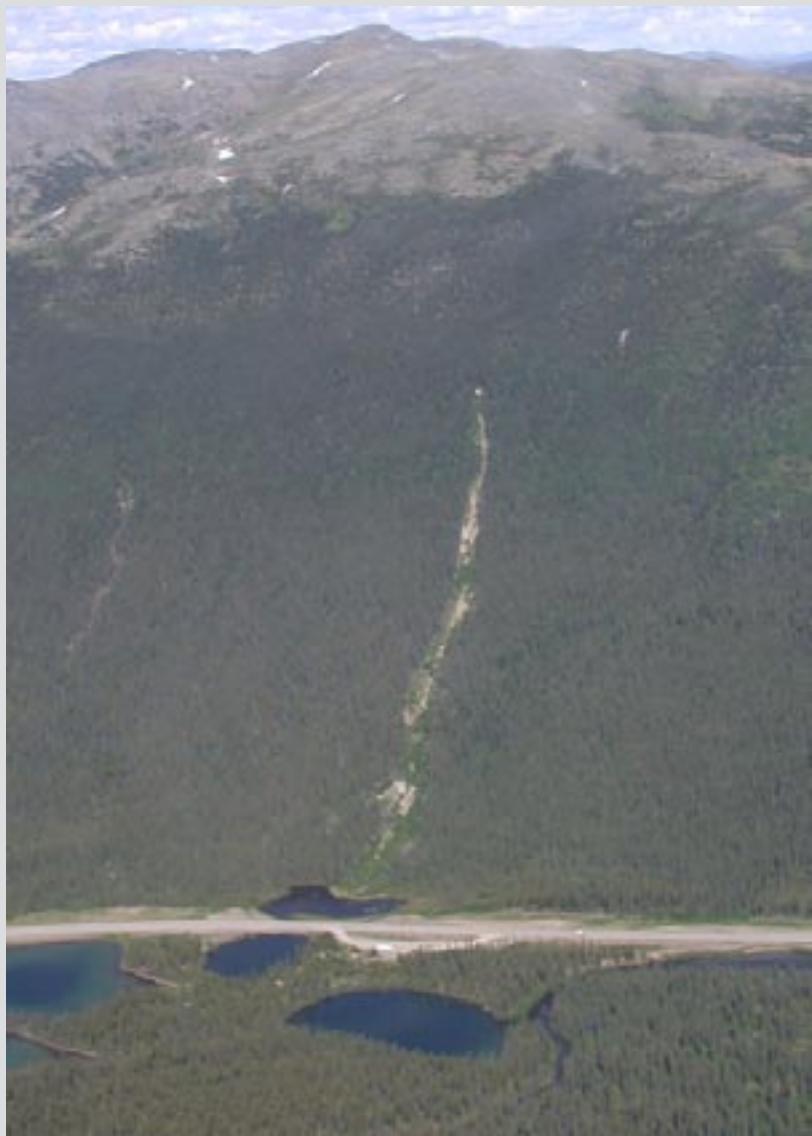
Figure XXII. Debris flow induced by intense rainstorm in 1988 on south-facing slope near Rancheria Message Post. Alaska Highway in foreground.
