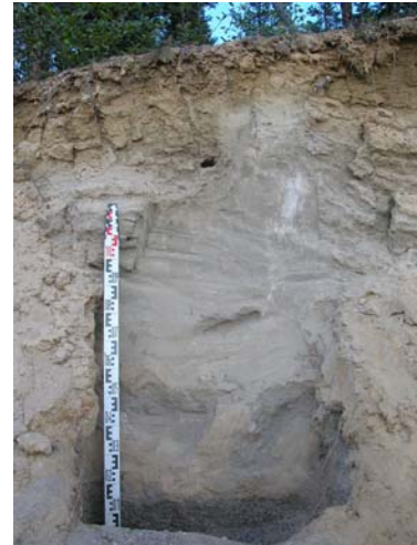
Figure 17. Fine sands and silts showing load deformation near base, just above glaciofluvial gravels in gravel pit (site 04WL128).
