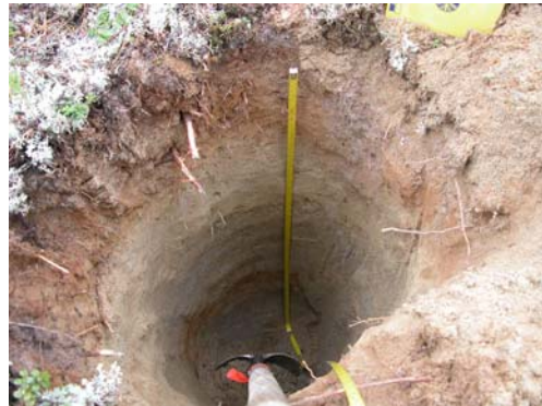
Figure 5. Typical soil pit (90 cm deep) for site soil and terrain classification. Pit is dug in hummocky glaciofluvial terrain (sgFGh-H). Site 04WL098.
