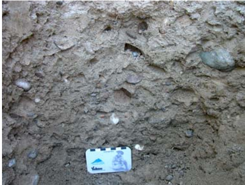
Figure 19. Typical structure of sandy basal till in Watson Lake area (site 04WLI25).
