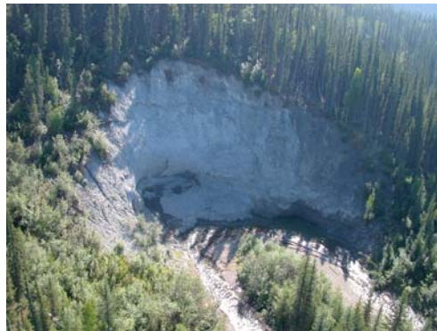
(B - right) Stiff glaciolacustrine clays at base of stream exposure.
