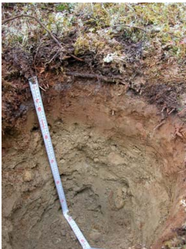
Figure 7. Typical soil pit (55 cm deep) in till, with 15 cm of oxidized loess at top (site 04WL175).
