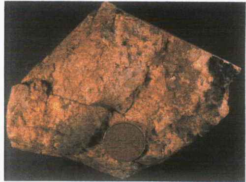
Plate 9. Pegmatite vein with anomalous tantalum levels (27 ppm). Great Horn MINFILE occurrence (105M 040).
