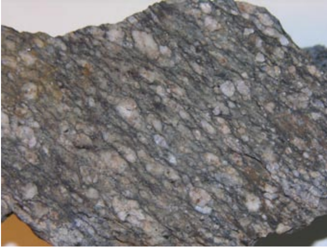
Figure 1-1. Protomylonitic fabric in granite of the Cassiar batholith near Rancheria Falls. Field of view is approximately 10 cm.
