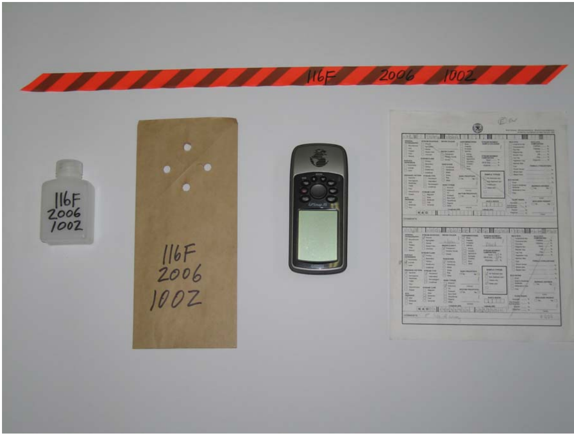
Figure 3. Example of pre-labelled flagging tape, Kraft paper bag, plastic bottle, Garmin GPSmap 76 and field card.
