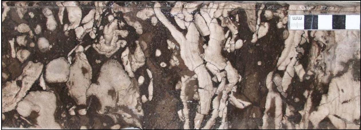
Figure 84. Core of Ramparts Formation Hume River D-53, about 507 m depth. Note oil stained matrix in floatstone packstone. Top of core is to left, scale card divisions in cm.
