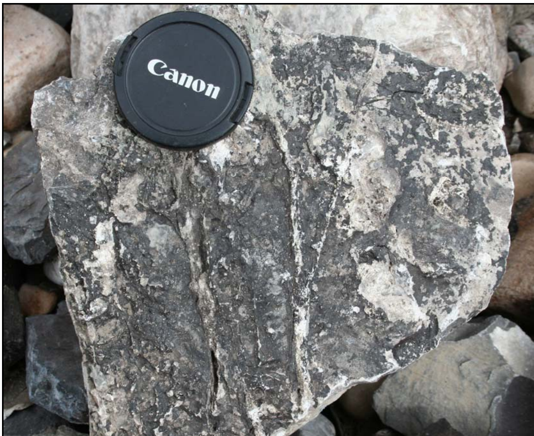
Figure 93. Float sample of Ramparts Formation, Powell Creek. The rock is oil stained, the surface shown here is bitumen coated, and calcite-filled fractures cut the rock.
