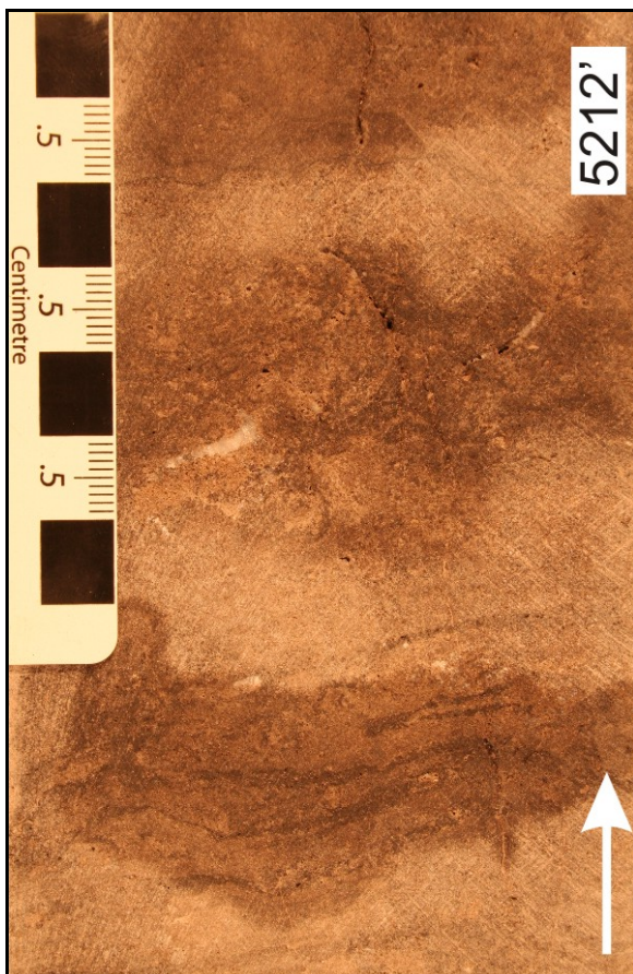
Figure 72. Outcrop of Arnica Formation sucrosic dolostone with intercrystalline porosity.
