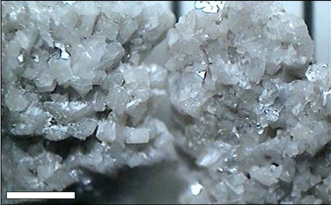
Figure 74. Well cuttings sample from Ontaratue K-04 well, 984.8m (3230 ft) in Arnica Formation. Sucrosic dolostone with good intercrystalline porosity. White scale bar is 1 mm.
