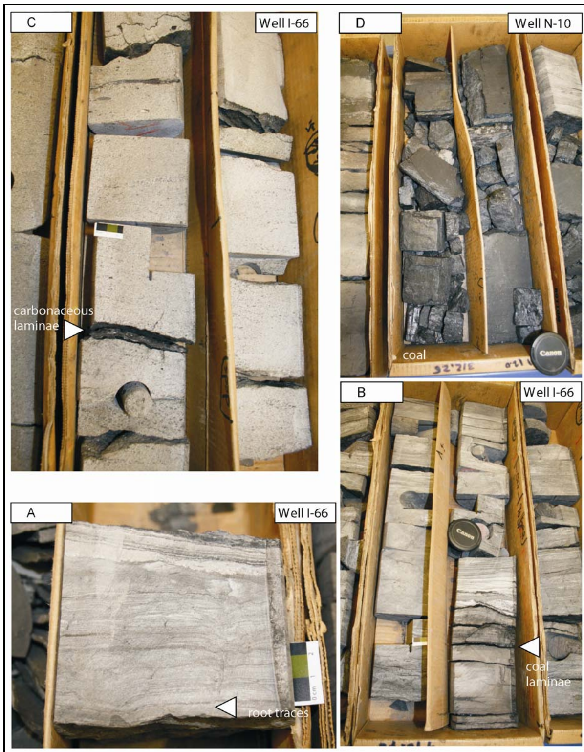
Figure 9.3.3. Photographs of Tukweye member from Hume River I-66 drill core: (A) root traces from floodplain facies; (B) coal laminae; (C) medium- to coarse-grained, trough cross-stratified sandstone interpreted as fluvial; and (D) 1.5 m thick coal bed from East Hume River N-10 drill core.
