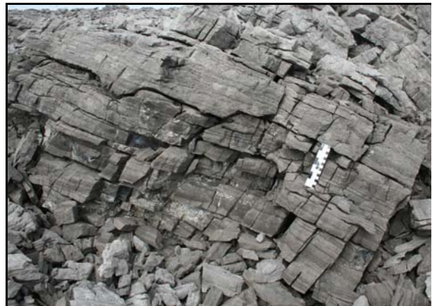
Figure 18. Laminated dolomudstone in middle unit of Mount Kindle Formation, Section LG-A1 (scale bar in cm and inches).
