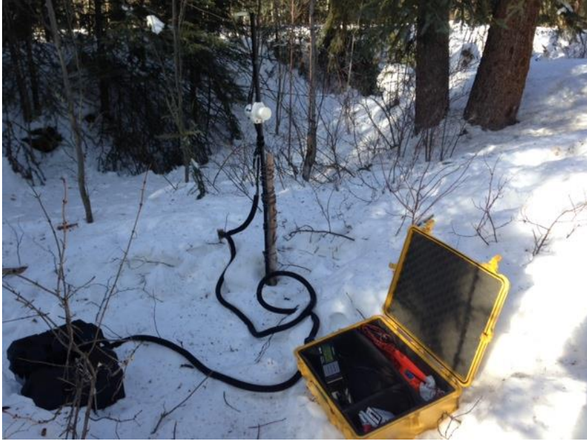
Figure 4 - Base Magnetometer Installation
