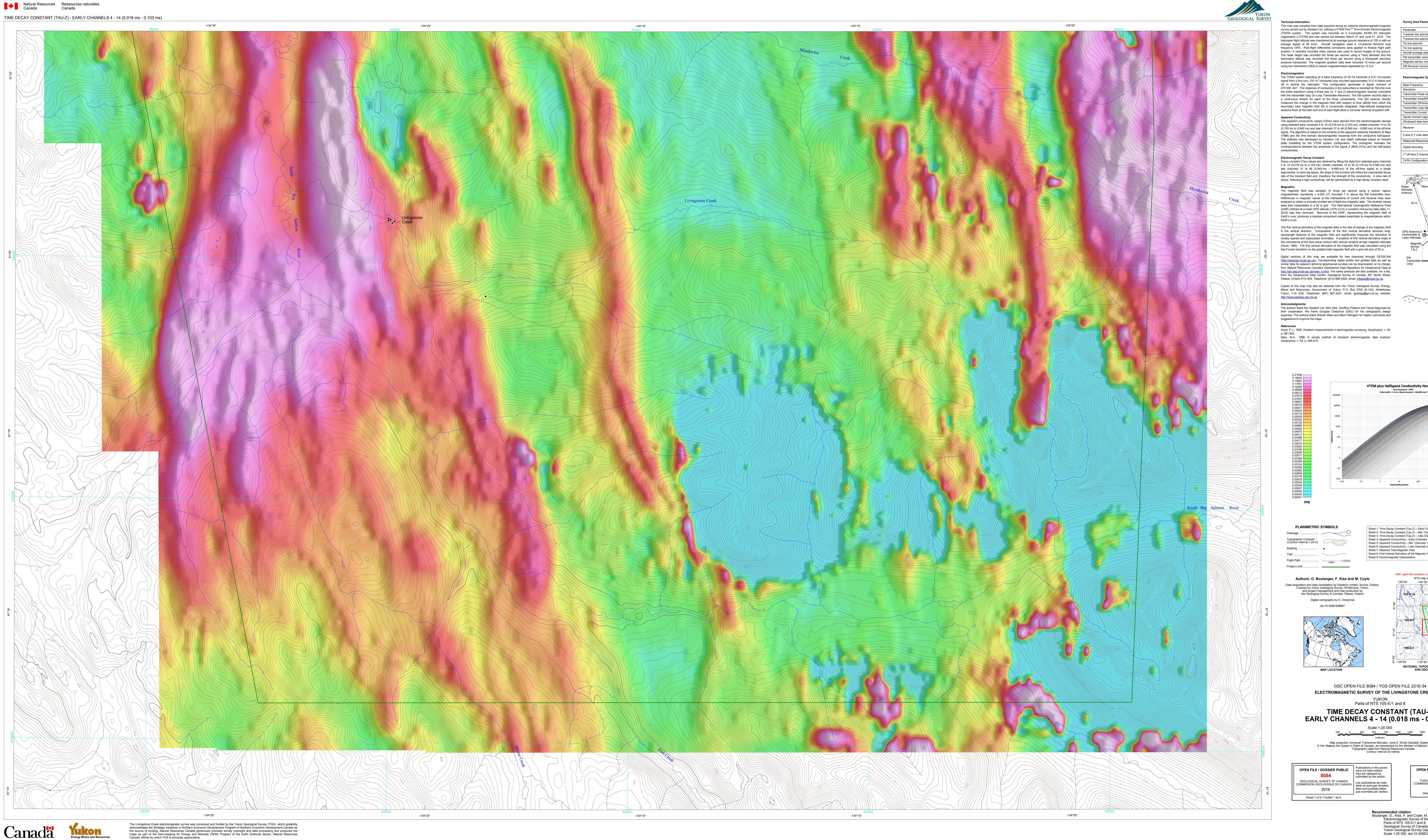
This map was compiled from data acquired during an airborne electromagnetic/magnetic survey carried out by Geotech Ltd. utilizing a VTEM Plus<sup>™</sup> Time-Domain Electromagnetic (TDEM) system. The system was mounted on a Eurocopter AS350 B3 helicopter (registration C-FVTM) and was carried out between March 31 and June 21, 2016. The helicopter flight altitude was maintained at an average ground clearance of 132 m with an
