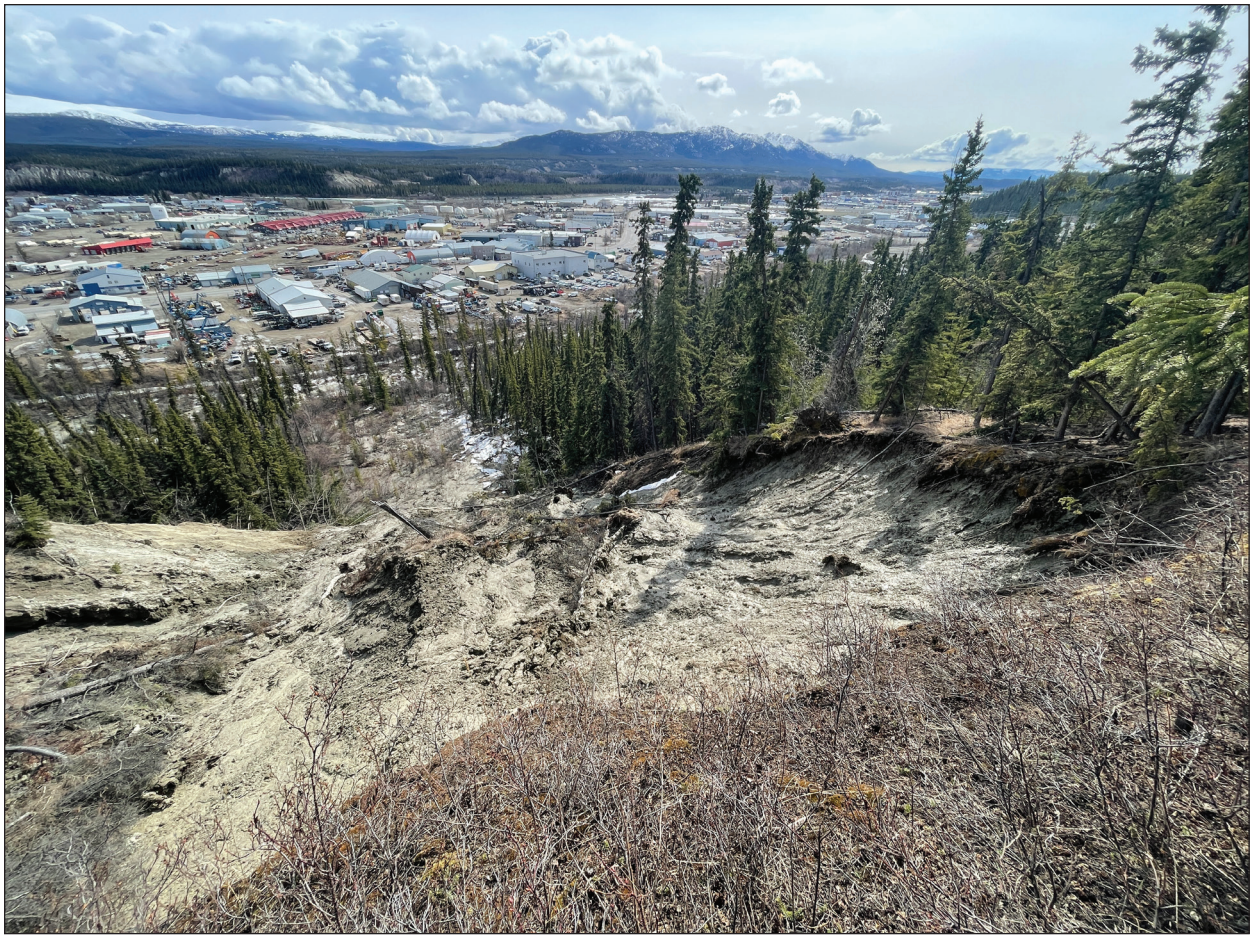
Figure 31. The headscarp area of the July 2000 Takhini East slide continues to actively retreat (May 5, 2022 photo).
