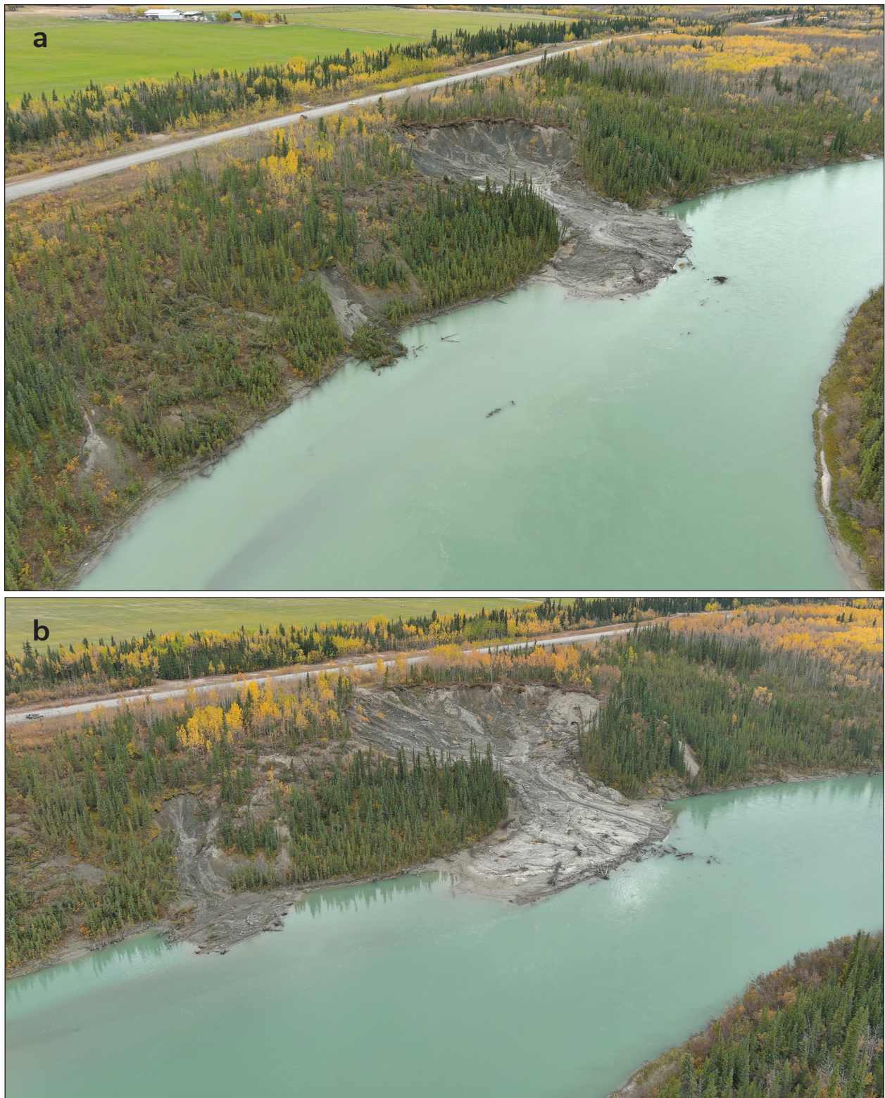
Figure 26. Oblique UAV photos of Takhini River retrogressive thaw flow, September 21, 2021 ( a ) and September 21, 2022 ( b ); Peter von Gaza photos. View is to the southwest, looking upstream; note vehicle on highway for scale ( a ). The thaw flow initiated in 2014 as a small failure similar in size to the one in the lower left corner of the upper photo. This smaller slide initiated as an active layer detachment in September 2021, and transitioned into a retrogressive thaw flow the following year.
