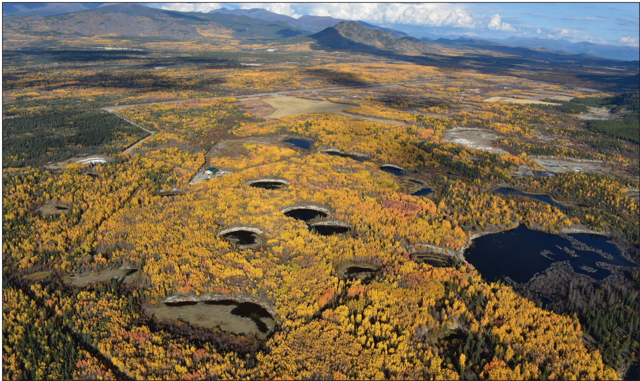
Figure 49. Thermokarst ponds are abundant in the Ibex Valley agricultural area, and are an excellent indicator of degrading ice-rich permafrost (17DA01-17DA04).
