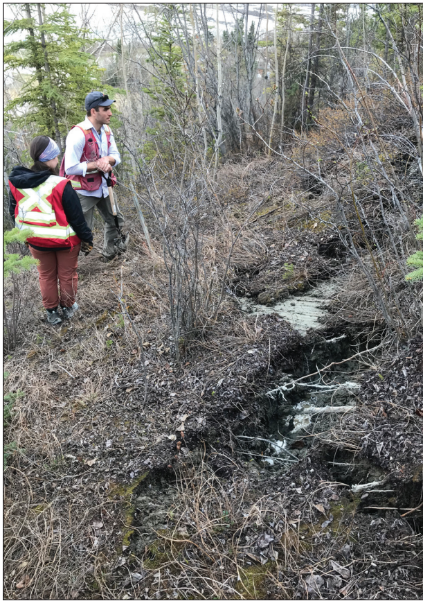
Figure 44. Indicators of active slope instability include fresh tension cracks, often spanned by outstretched roots (left) and split trees (right). May 2022 photo taken just south of slide in the Takhini East subdivision.
