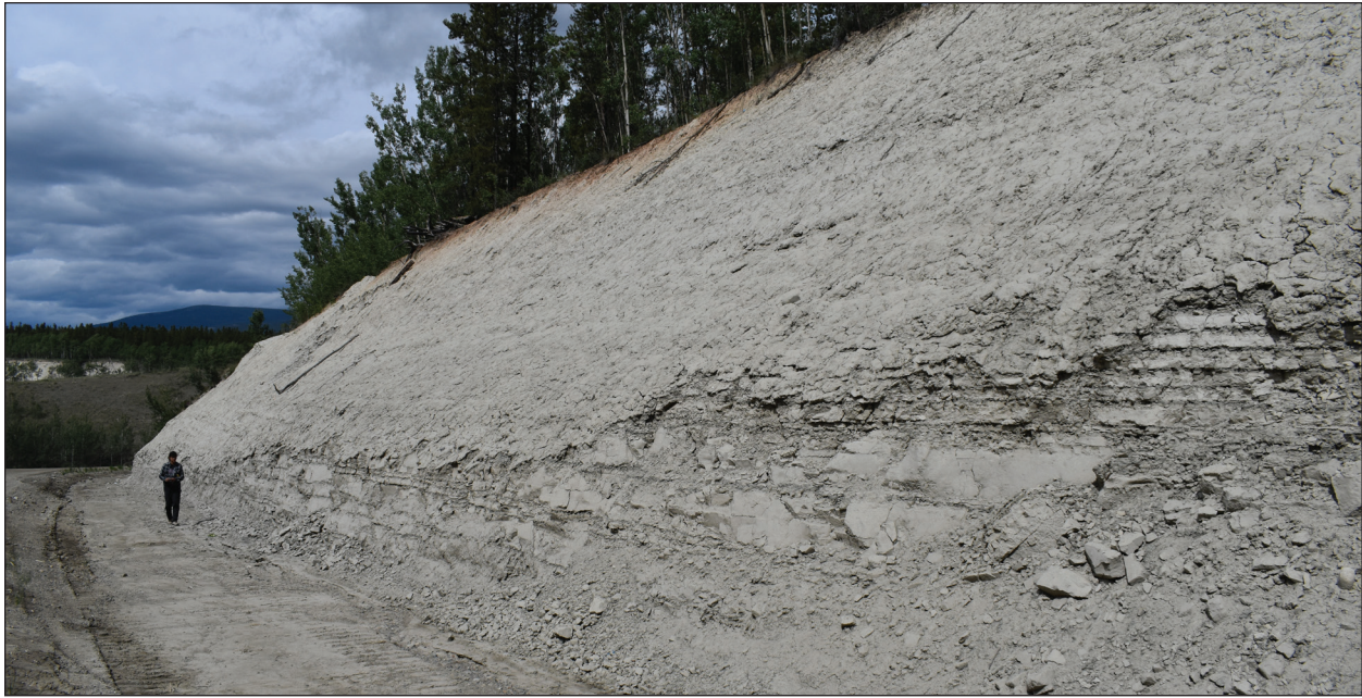
Figure 15. Glaciolacustrine sediments exposed in a roadcut along Takhini River Road (18PL074) consist of horizontally laminated layers of silt (thicker, lighter coloured layers) and clay (thinner, darker coloured layers up to approximately 5 cm thick). These sediments are easily eroded and are subject to gullying and piping in this area.
