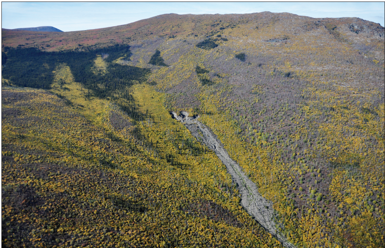
Figure 25. This landslide occurred in May 2010 on the eastern flanks of Haeckel Hill. The slide adversely impacted water quality in Little Takhini Creek. Approximately 10 m of till was exposed in the headscarp. While permafrost was not confirmed in the headscarp, the morphology and site characteristics suggest it is a retrogressive thaw flow. September 2010 photo by Cameron Eckert.
