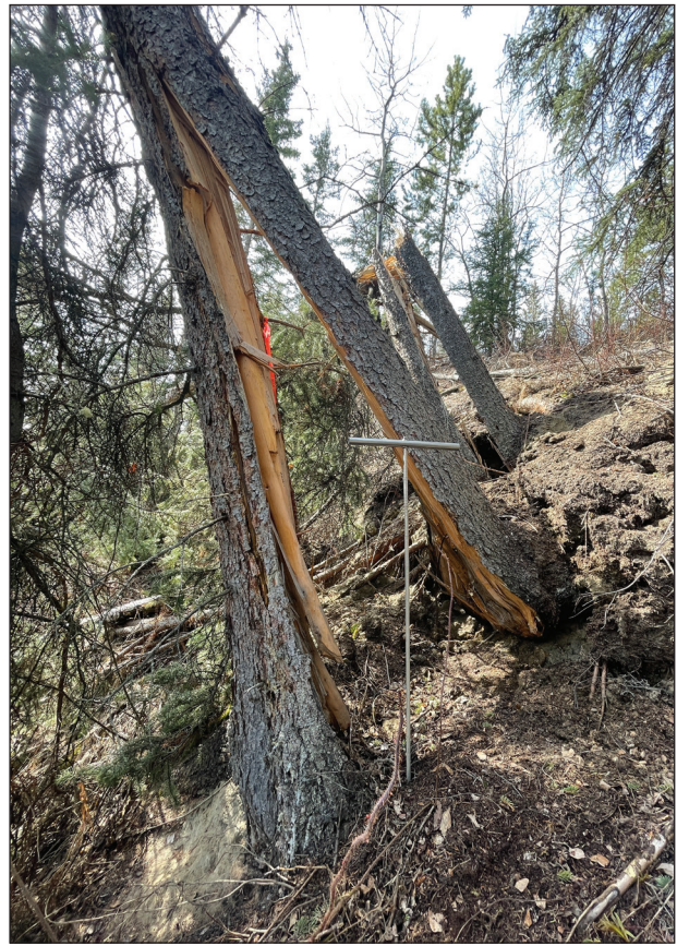
Figure 44. Indicators of active slope instability include fresh tension cracks, often spanned by outstretched roots (left) and split trees (right). May 2022 photo taken just south of slide in the Takhini East subdivision.
