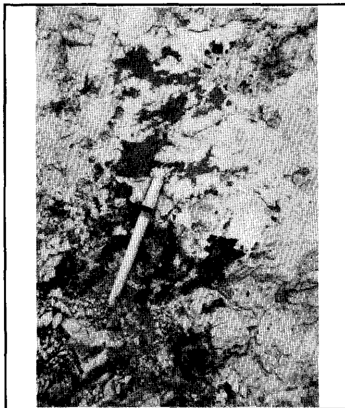
Figure 1. Irregular patches of coarse grained galena and red sphalerite in massive barite.
