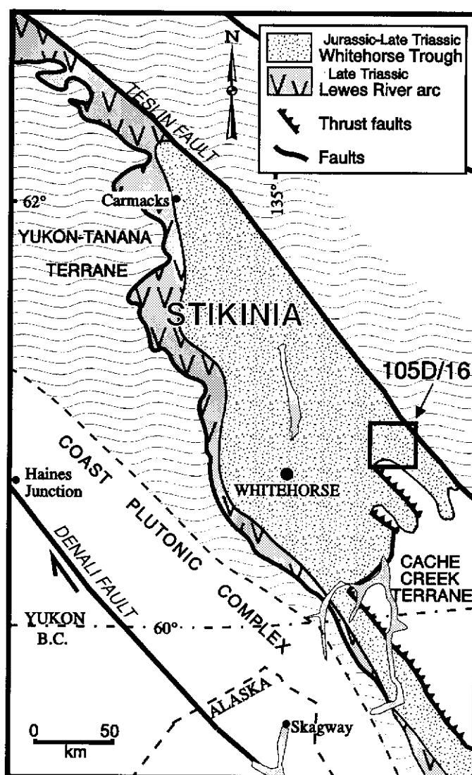
Figure 2: The regional tectonic setting of southern Yukon with the map area outlined. The map area is underlain primarily by the Whitehorse Trough rocks of Stikinia but also includes small portions of Cache Creek and Yukon-Tanana Terrane.
