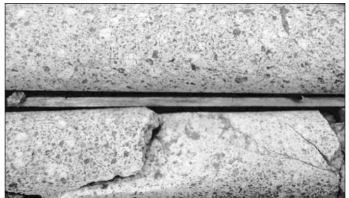
Figure 3. Diamond drill core (NQ-size) of the Tad porphyry from the oxide zone. Light-coloured phenocrysts are quartz and alkali feldspar; dark specks are altered plagioclase.
