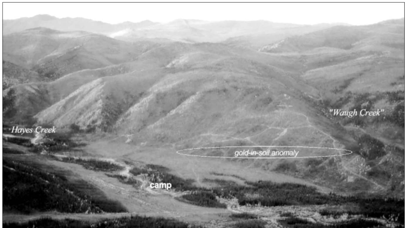
Figure 4. View southwesterly over the Tad property, showing the location of the gold-in-soil geochemical anomaly identified by Noranda in 1987. This anomaly likely represents the intersection of supergene gold horizon with the present erosion surface.
