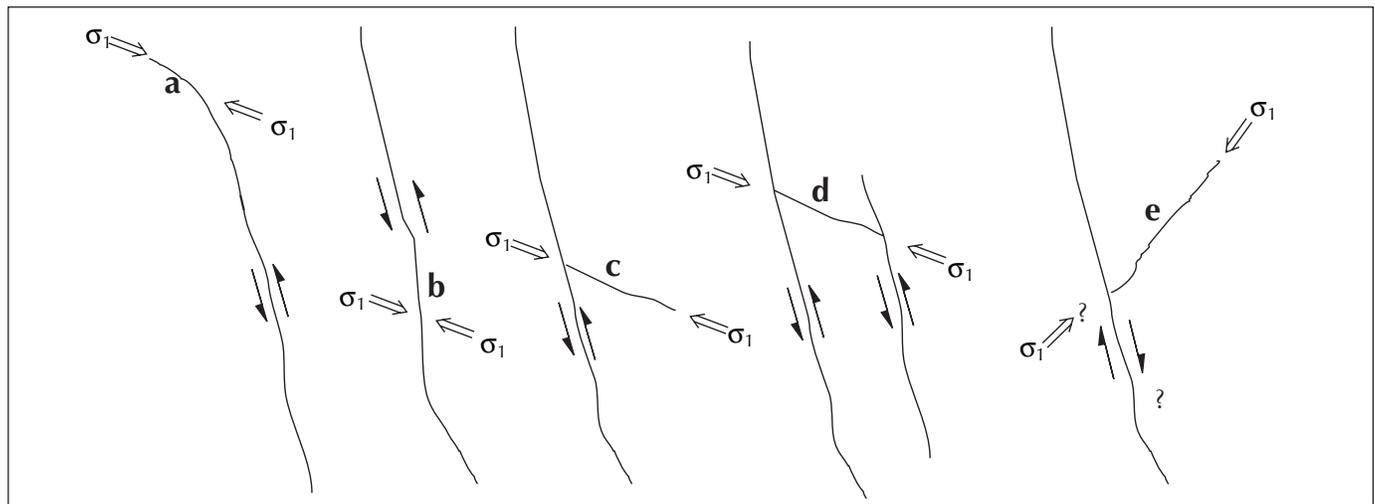
**Figure 9.** Favourable structural sites for mineralization a) favourably misoriented segment of BF<sub>a</sub> fault b) unfavourably misoriented segment of BF<sub>a</sub> fault c) BF<sub>b</sub> fracture zone linked to BF<sub>a</sub> fault d) BF<sub>b</sub> fracture zone linking two BF<sub>a</sub> faults e) BF<sub>c</sub> fracture zone connected to BF<sub>a</sub> fault, perhaps with dextral movement.
