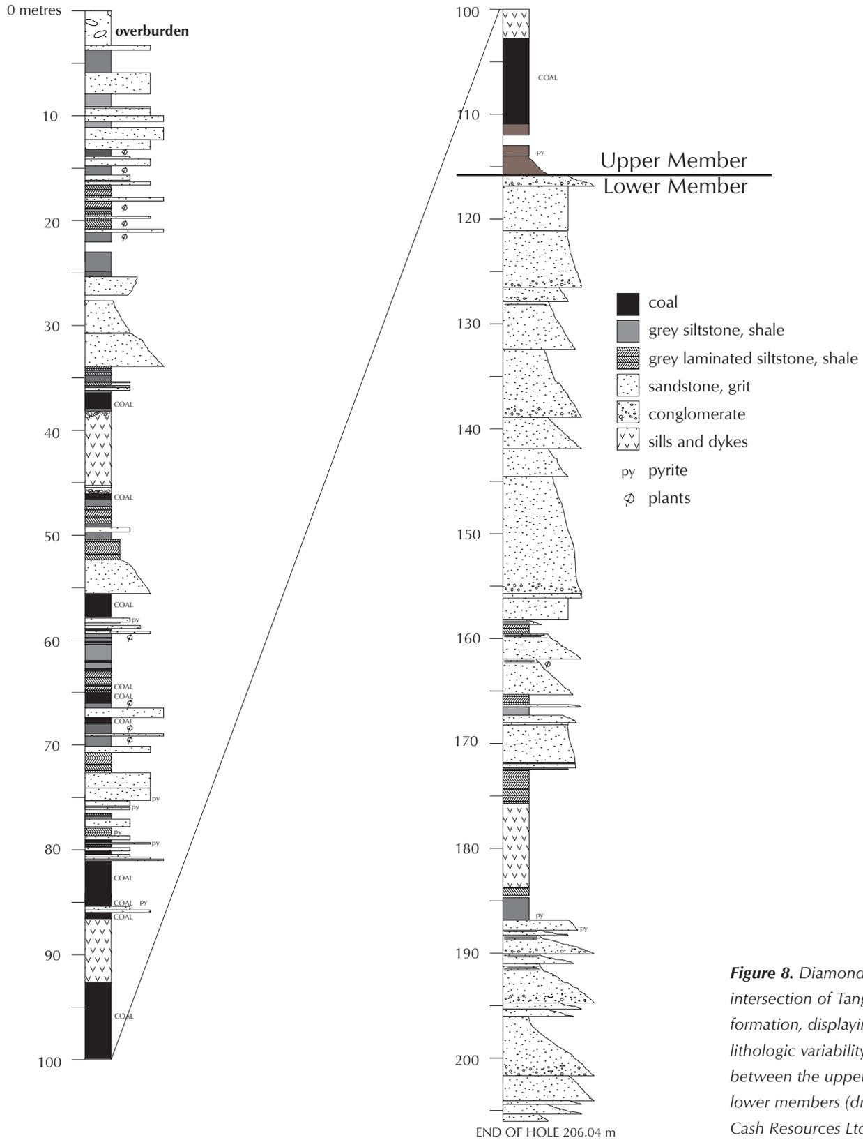
**Figure 8.** Diamond drill hole intersection of Tanglefoot formation, displaying lithologic variability between the upper and lower members (drilled by Cash Resources Ltd.).
