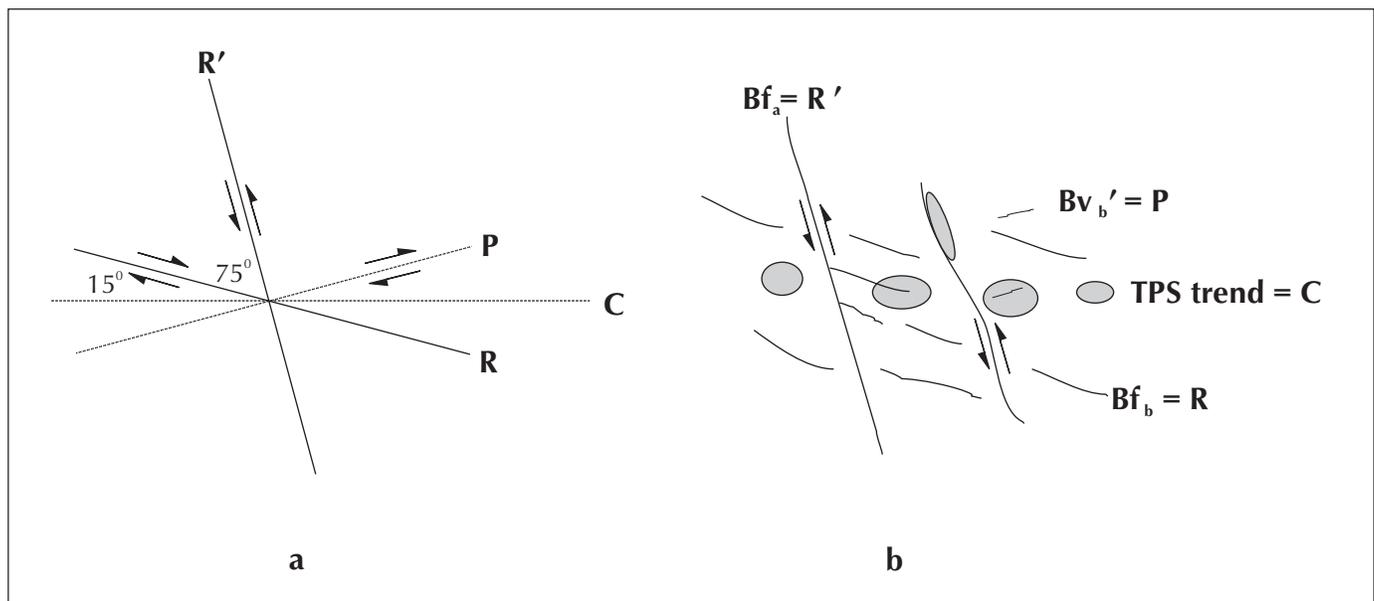
**Figure 14.** Possible application of a Riedel shear model to the Clear Creek area. *C* is represented by the E-W trend of the TPS belt, *R'* is represented by  $BF_a$  sinistral faults, *R* is represented by  $BF_b/BV_b$  fracture zones and veins, *P* is represented by the subset  $BV_b'$  (only observed at outcrop scale).
