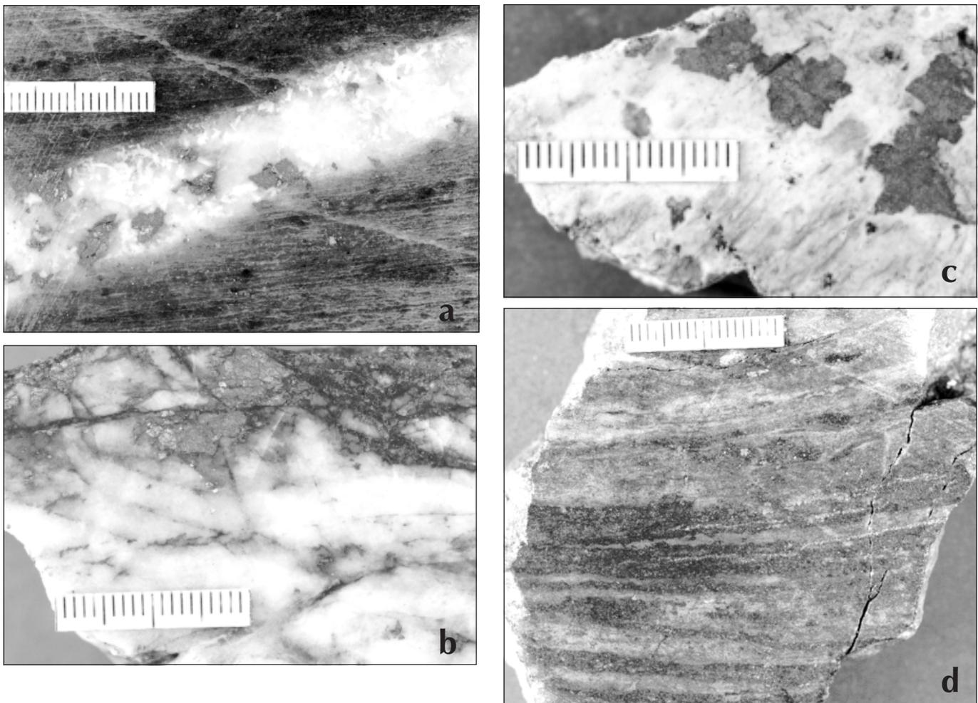
**Figure 5.** Styles of gold mineralization at Scheelite Dome: a) quartz-arsenopyrite extension veins; b) typical fault-vein material displaying crack seal textures (stibnite is concentrated along fractures in the quartz-arsenopyrite assemblage); c) disseminated arsenopyrite in sericitized quartz-phyllite; and d) folioform replacement of calc-silicate rock by pyrrhotite, lesser arsenopyrite, and minor chalcopyrite.
