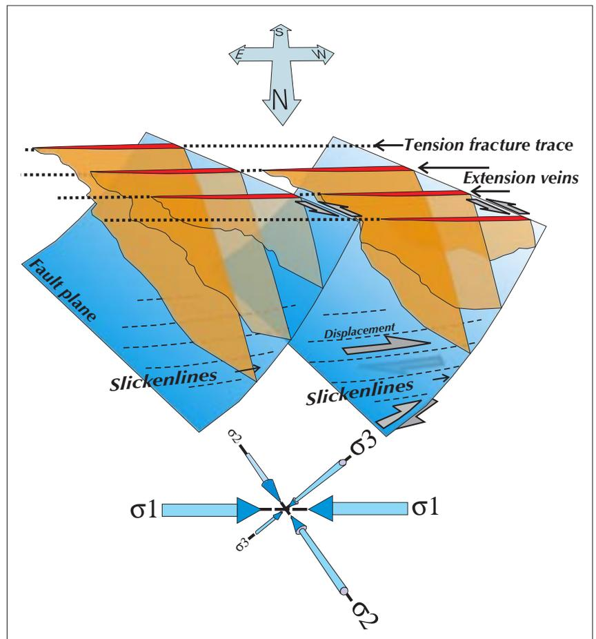
**Figure 7.** Schematic depiction of the key structures controlling mineralization and the inferred orientation of the far-field stress regime at the time (view toward the south). Note, extension veins are best developed in the hanging walls of northwest-trending faults.
