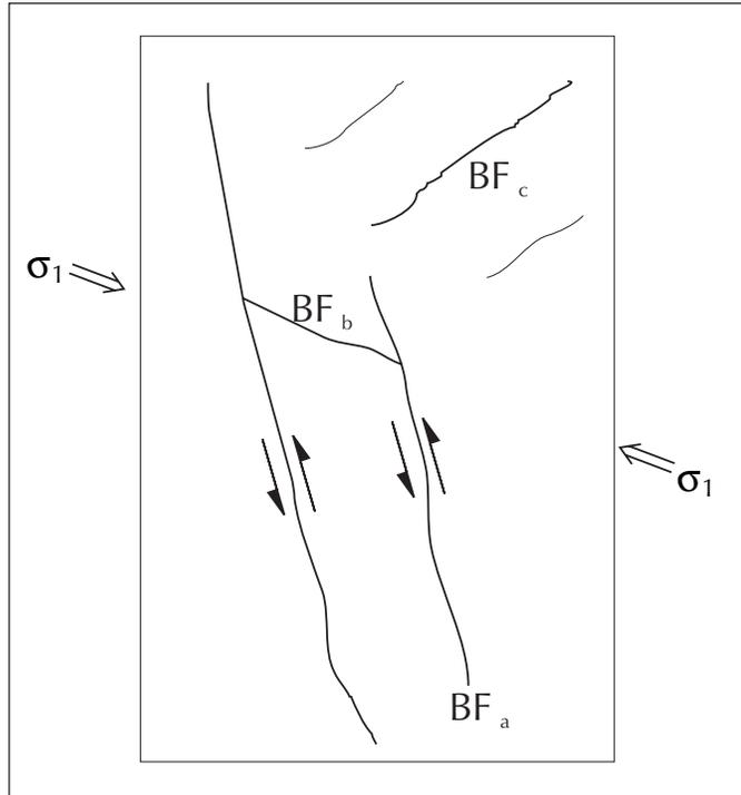
**Figure 8.** Schematic sketch of the major fault/fracture types at Clear Creek. BF<sub>a</sub> are strike-slip faults, BF<sub>b</sub> are transtensional and BF<sub>c</sub> are transpressional faults.
