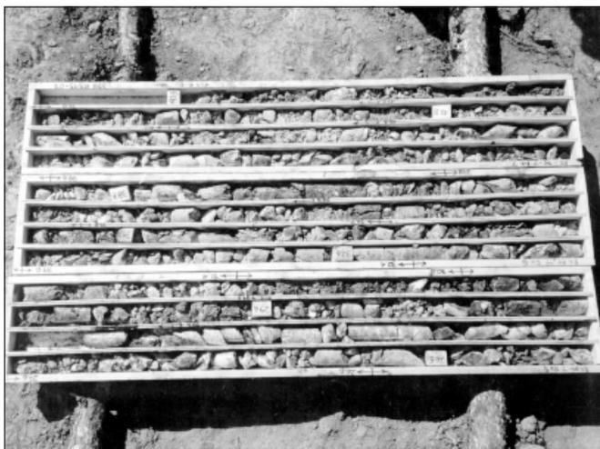
**Figure 13.** Typical broken and crumbly nature of clay-rich and limonitic supergene-altered mineralization at Rusty Springs in drill core. In this case the mineralized zone represents discordant material from Mike Hill, but it is similar in general appearance and mineralogy (though of higher grade) to typical Katshat unit mineralization. DDH95-07: 15.3 m assaying 518 g/t Ag, 0.77% Pb, 3.0% Cu, and 1.3% Zn.
