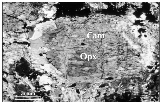
**Figure 9.** Photomicrograph of gabbronorite. The original orthopyroxene (Opx) is almost completely replaced by clin amphibole (Cam) and only preserved as a relic in the centre of the crystal. Scale bar: 0.5 mm. XPL.
