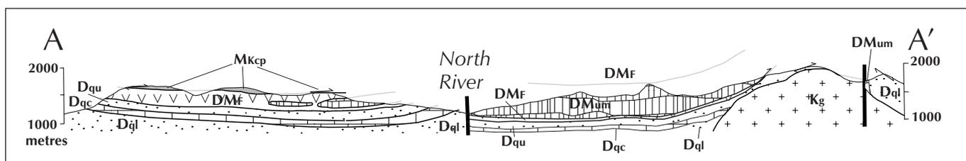
**Figure 5.** Cross-section along line A-A' shown in Figure 2. Legend as in Figure 2. Thickness of unit D<sub>qc</sub> east of the North River is not known with certainty. The lower and upper parts of unit D<sub>q</sub> are indicated as units D<sub>ql</sub> and D<sub>qu</sub>, respectively.
