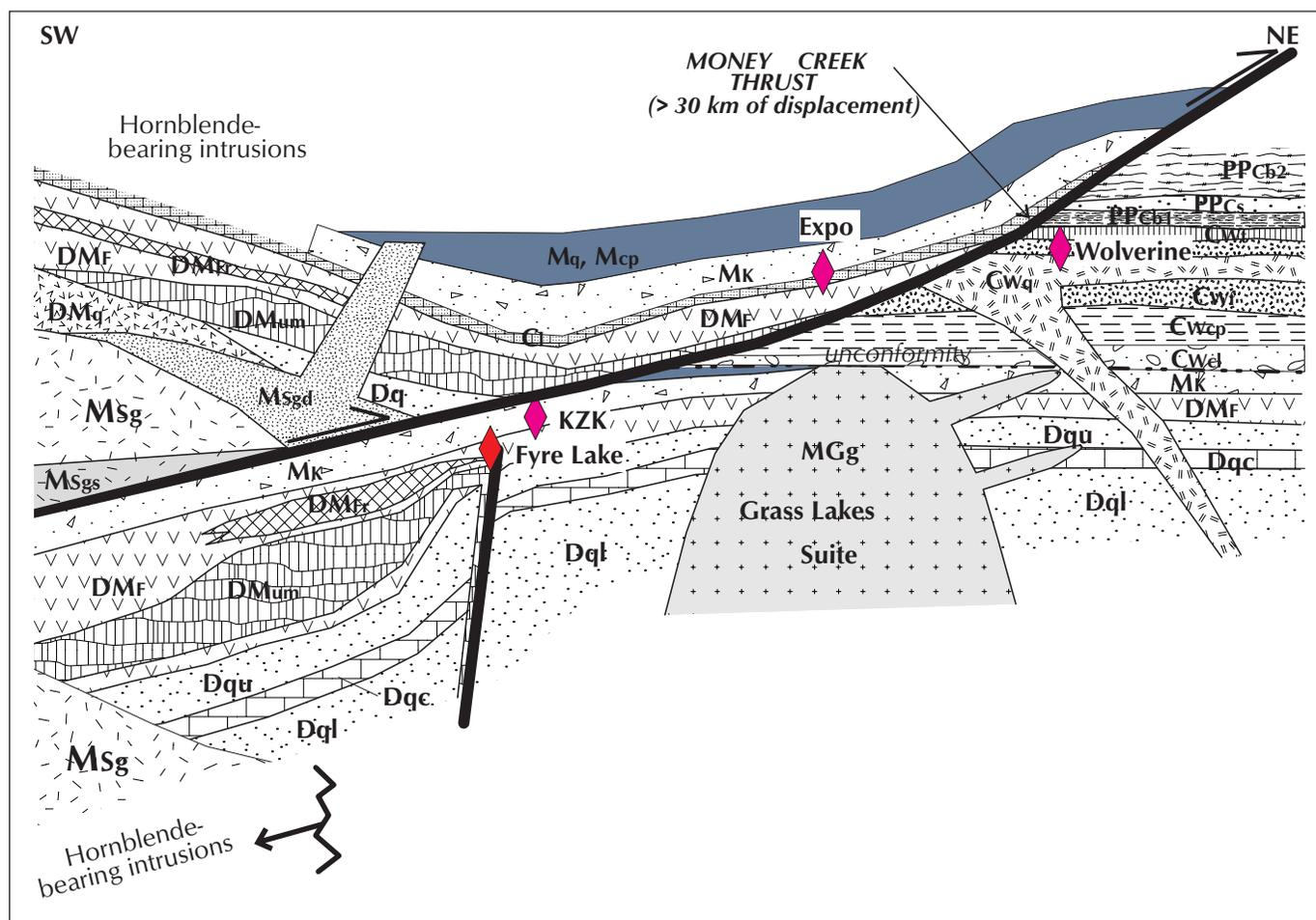
**Figure 12.** Schematic northeast-southwest cross-section summarizing the stratigraphy and intrusive rocks in the hanging wall and footwall of the Money Creek thrust sheet. Legend as in Figure 2. The appearance of hornblende-bearing granitic meta-plutonic rocks in the footwall near the Tintina Fault is indicated schematically by the jagged vertical line. KZK = Kudz Ze Kayah.
