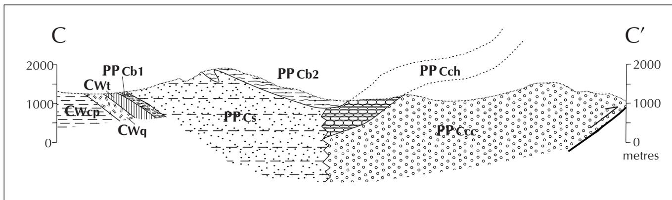
**Figure 8.** Cross-section across Campbell Range along line C-C' in Figure 7. Legend as in Figure 2. In this figure, unit PPCs, on the northeast side of the Campbell Range, is subdivided into a lower unit PPCcc and an upper unit PPCch. See text for discussion.
