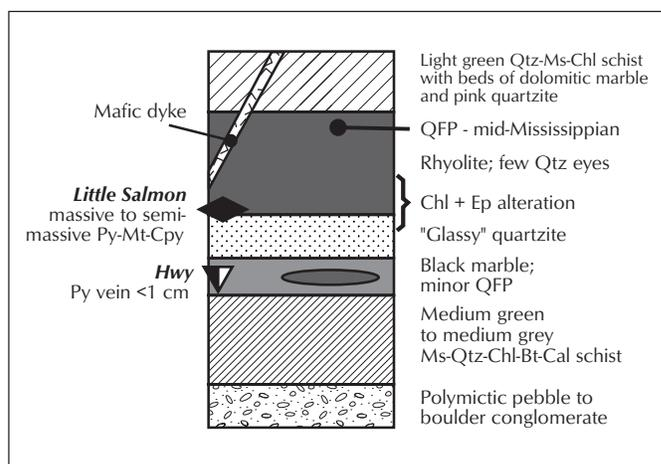
**Figure 8.** Detailed stratigraphy of the base of Unit 3 near the Little Salmon occurrence, along the west flank of the Little Salmon volcanic sequence. Stratigraphic position of mineral occurrences are indicated. QFP = quartz-feldspar porphyry, Qtz = quartz, Ms = muscovite, Chl = chlorite, Ep = epidote, Bt = biotite, Cal = calcite, Py = pyrite, Mt = magnetite, Cpy = chalcopyrite.
