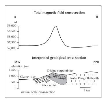
**Figure 3.** Magnetic field cross-section and interpreted geological section through the Doghead Point ultramafic body. The subsurface extension of the serpentinite is speculative. See Figure 2 for location of section.
