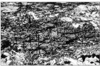
*Figure 5.* Enlarged view of the lower right section of Figure 4 showing the web-like alteration of olivine. Scale bar: 0.5 mm. XPL.
