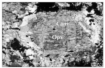
**Figure 9.** Photomicrograph of gabbronorite. The original orthopyroxene (Opx) is almost completely replaced by clinoamphibole (Cam) and only preserved as a relic in the centre of the crystal. Scale bar: 0.5 mm. XPL.
