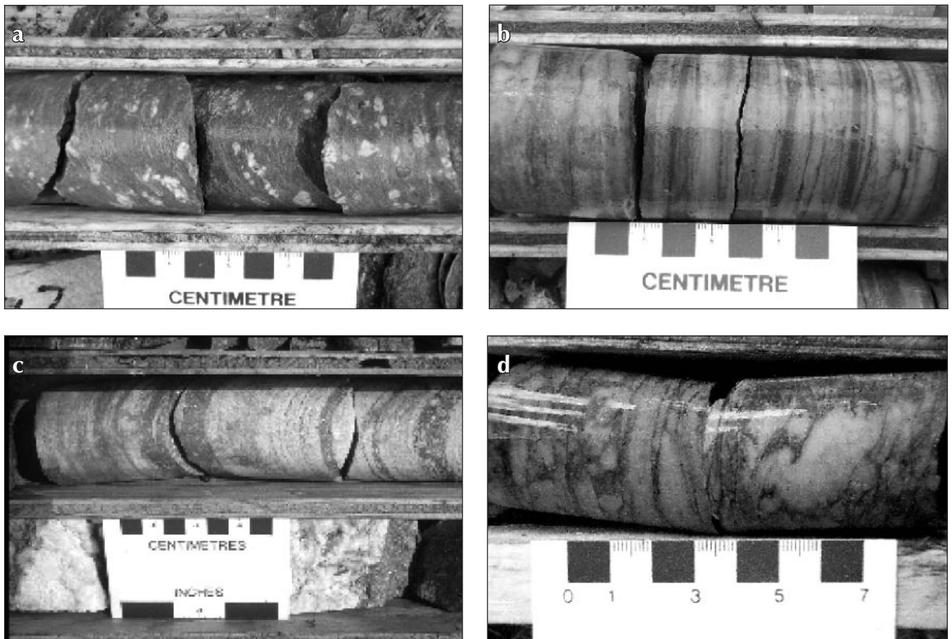
Figure 8. Photographs of host-rock lithologies: (a) K-feldspar-pyric rhyolite porphyry of Unit 1; (b) magnetite exhalite (iron formation) of Unit 2; (c) carbonate-pyrite exhalite of Unit 2; and (d) fragmental rhyolite of Unit 3.
