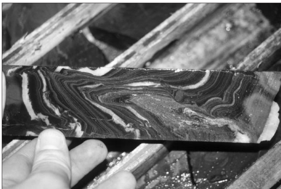
Figure 15. Banded sphalerite-galena mineralization showing de-watering structures from Hole A-67 drilled in the Don Valley area at the Howards Pass project.
