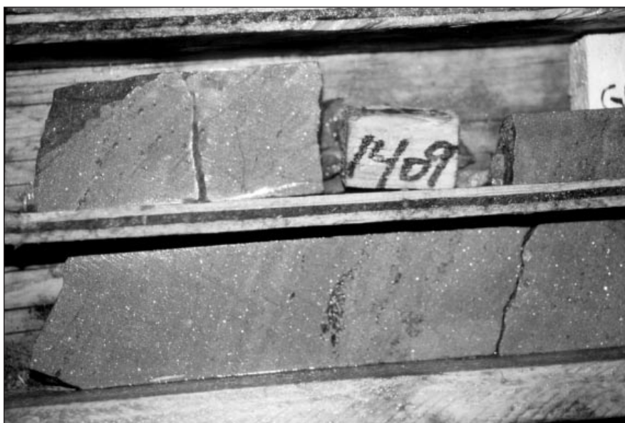
Figure 9. Close-up of massive sulphide intersection from drill hole WW00-01 on the Wolverine project (NQ core). The hole intersected 7.4 m of 13.56% Zn, 1.16% Pb, 0.68% Cu, 152 g/t Ag and 0.59 g/t Au.
