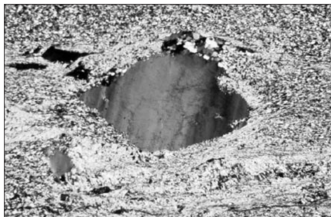
Figure 5. Thin section of angular quartz eye in felsic metavolcanic unit. Field of view = 7.2 mm.
