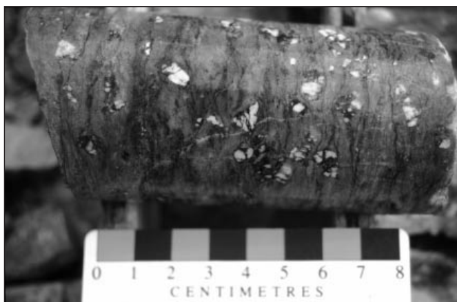
Figure 8. Puck zone feldspar porphyritic intrusion with variably broken K-feldspar grains with partial replacement by secondary K-feldspar.
