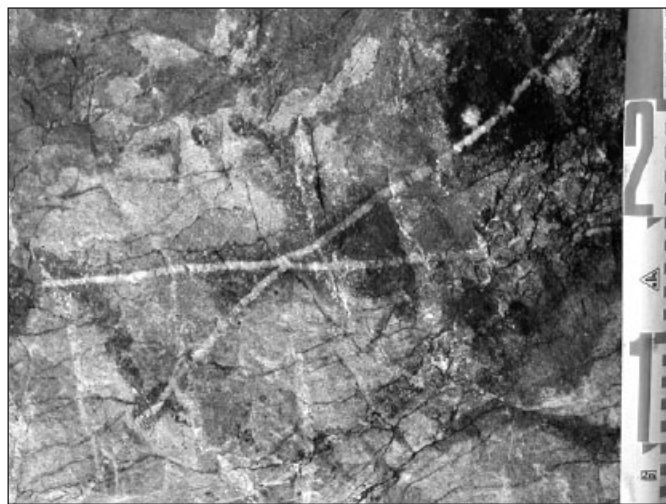
Figure 4. Quartz stockwork with tourmalinization (dark patches) along selvage and along fractures. The sericitized-quartzite host rock is pale in colour. Scale divisions are in centimetres.
