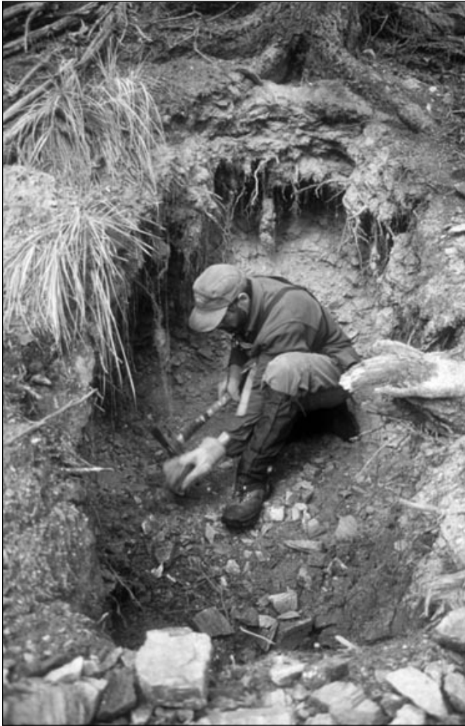
Figure 7. Shawn Ryan is seen here in a pit located on the Ryan Creek anomaly where C horizon soils returned values of up to 1.19% Cu.
