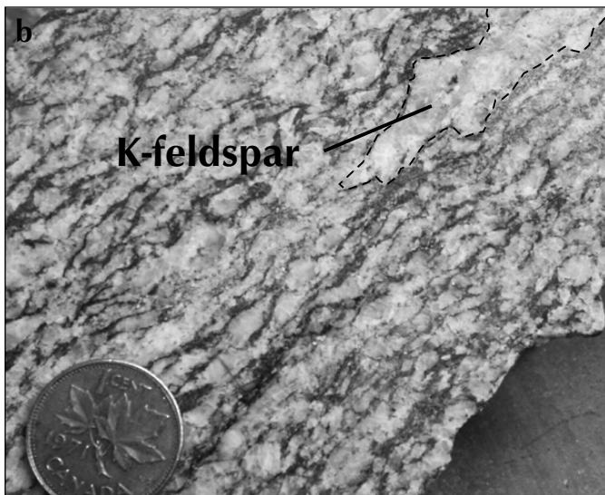
Figure 3. Representative igneous rock units from Minto: (a) typical massive, K-feldspar-phyric hornblende-biotite granodiorite (phase 2) of the Granite Mountain Batholith; (b) strongly foliated and weakly mineralized biotite granodiorite meta-intrusive rock with broken and strung-out K-feldspar phenocryst (phase 5).
