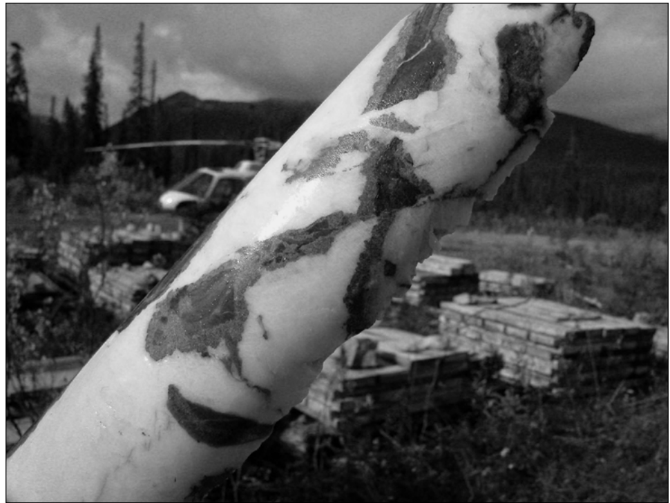
Figure 23. Sphalerite-galena mineralization in calcite-quartz breccia on Noranda's Andrew property.
