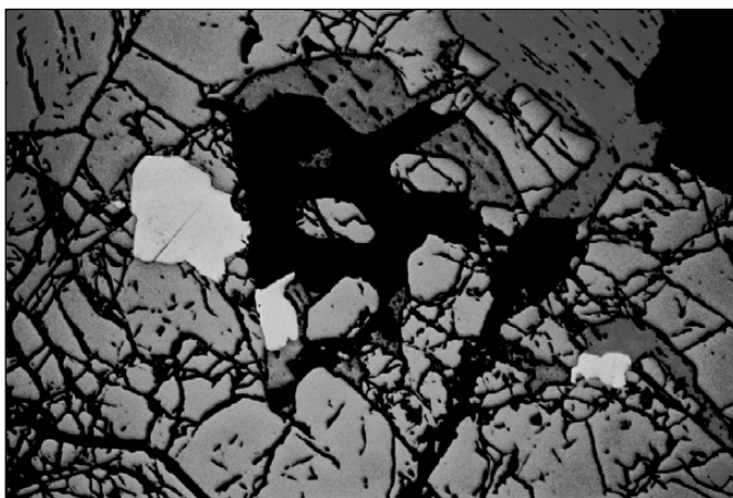
Figure 7. Photomicrograph that illustrates the paragenetic relationship between electrum (white) and late galena (darkest grey with larger black pits). Both minerals replace early, coarse-grained pyrite (medium grey) in a quartz-sulphide mineral extension vein. The largest electrum grain is about 200 microns across. Sample is from the 1300-level in the Rainbow zone. Reflected light, field of view 0.16 mm.
