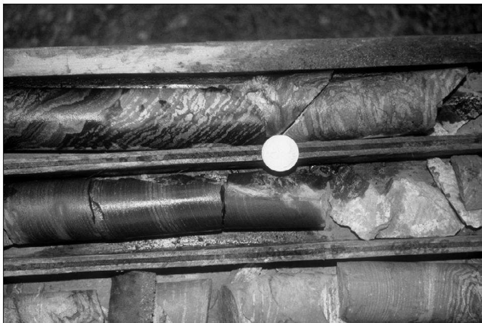
Figure 22. Bedded pyrite in black shales from the Tanner property of Manson Creek Resources.
