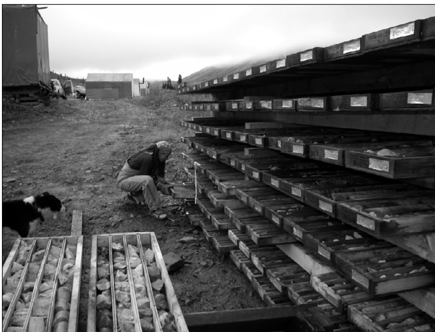
Figure 6. Anna Fonseca, geologist, examining drill core at Regent Ventures' Red Mountain project.
