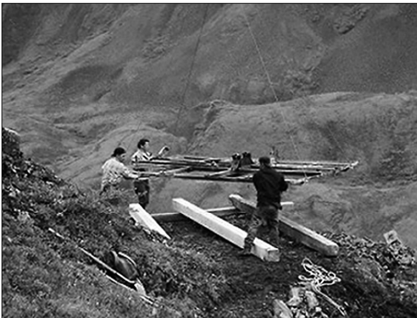
Figure 13. A helicopter gently moving the drill into place on the Arn claims. Note the small area affected by this method of drilling. Photo by Atac Resources.
