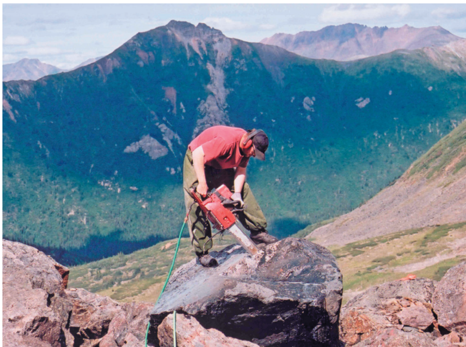
Figure 37. Diamond-impregnated chain saws were used for sampling at the True Blue property.
