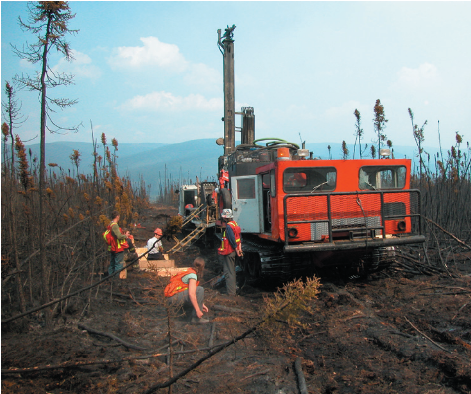
Figure 3. Boulder Mining Corporation's rotonomic drill in operation in the Indian River area in 2004. The drill was successful in recovering intact stratigraphic samples of gravel in core which was processed for heavy minerals and gold after detailed descriptions and documentation.
