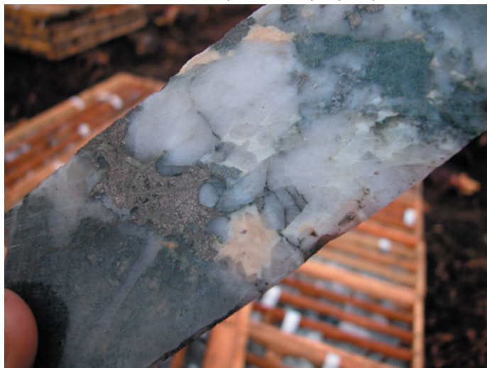
Figure 8. Quartz-carbonate mineral vein with pyrite-arsenopyrite from drilling at the Lynx Creek property.
