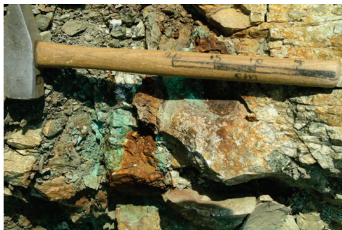
Figure 11. Photograph of area that sample 04-SIS-137-3-1 was taken from. Zone just below hammer in centre of photograph is composed of chalcopyrite, pyrite and malachite.
