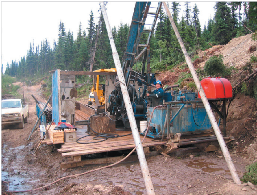
Figure 13. Diamond drilling on the Hyland Gold property.
