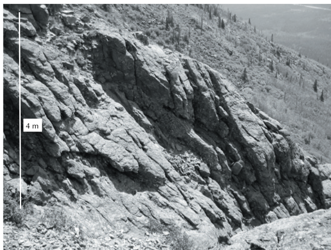
Figure 4. Dominant discontinuity set IV in the headscarp area of the Aishihik River landslide. Note the close spacing (60 to 200 mm) of the discontinuity set.
