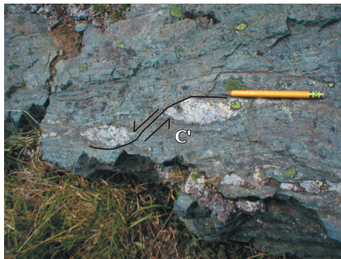
Figure 10. Extensional C' shears in mylonite on Tally Ho Mountain. The sense of movement indicated by the shears is top-down and to the east. Pencil parallels C fabric.
