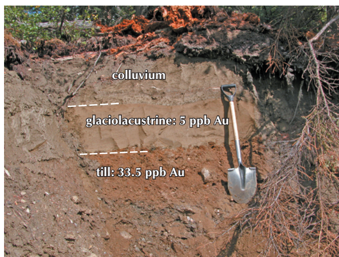
Figure 12. A surficial sediment profile in Seagull Creek valley showing a veneer of glaciolacustrine sand overlying a till. The gold concentrations from each unit show the geochemical variability within the surficial geology and highlights the need for surficial mapping early in the exploration process.
