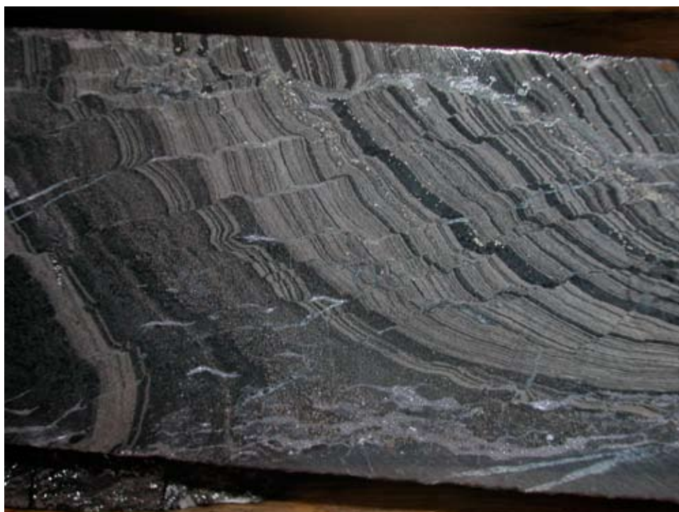
Figure 18. High-grade zinc-lead mineralization in drill core from the XY deposit at Howard's Pass.
