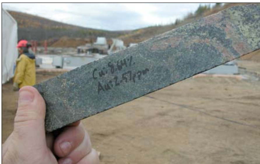
Figure 10. High-grade core from in-fill drilling on the Minto deposit.
