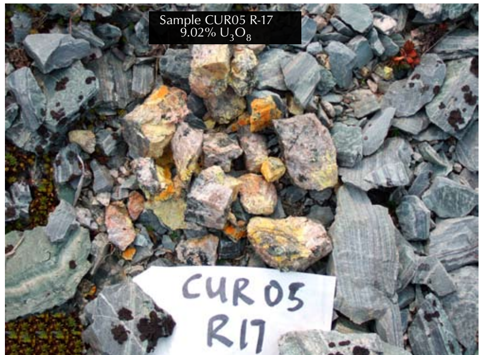
Figure 15. High-grade uranium in sheared and hydrothermally altered, quartz-feldspar-chlorite-veined, fine-grained sedimentary rocks at the Curie property. Photo by Aurora Geosciences.
