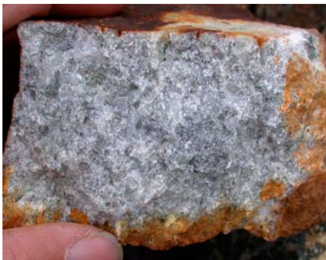
Figure 11. Siliciclastic Hyland Group grit from the Sprogge property with disseminated blebs of pyrite and arsenopyrite (dark grey) in the matrix.
