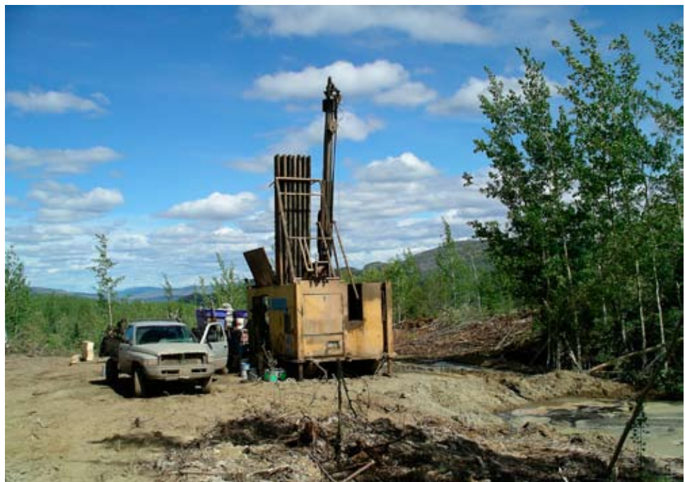
Figure 35. Diamond drill at the Division Mountain Coal project.
