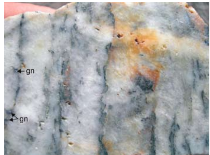
Figure 8. Ribbon-banded quartz veins separated by graphitic septa. Galena (gn) occurs along some of the septa. The rock is approximately 12 cm across.
