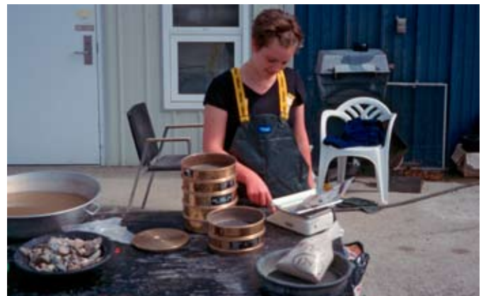
Figure 2. Gravel samples were dried and sieved through a series of US Standard mesh screens to determine matrix grain-size distribution.
