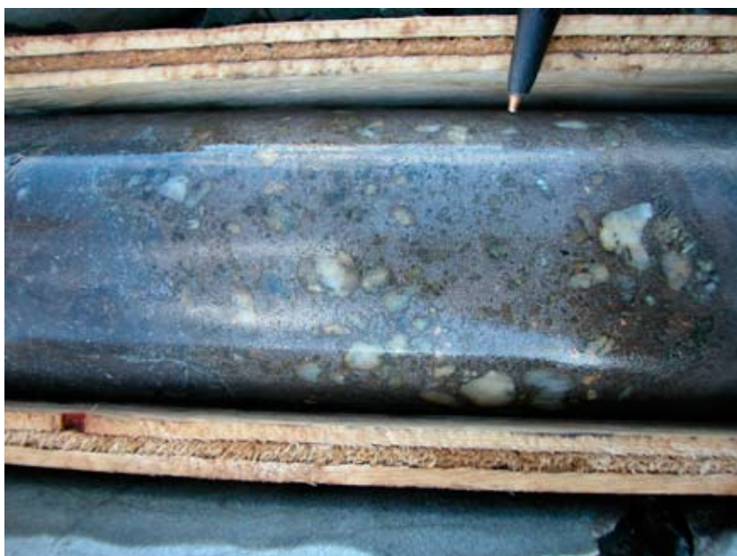
Figure 25. Massive pyrrhotite-pyrite manto-style mineralization from Ketz River.
