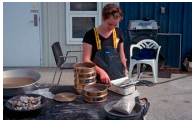
Figure 2. Gravel samples were dried and sieved through a series of US Standard mesh screens to determine matrix grain-size distribution.
