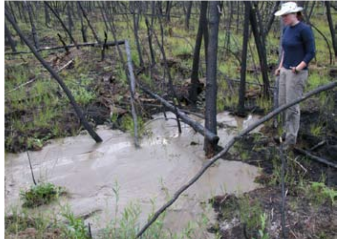
Figure 9. Surface sediment plume created by artesian groundwater flow. These commonly occurred on saturated slopes and near the initiation zones of recent failures.
