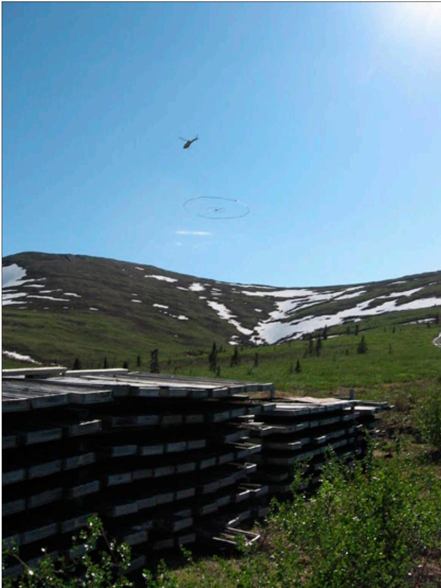
**Figure 14.** Versatile Time-Domain ElectroMagnetic (VTEM) surveying of the Red Mountain gold project of Regent Ventures.
