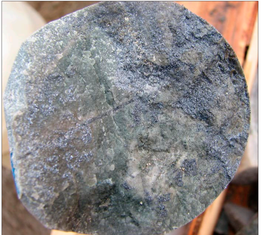
Figure 35. Molybdenum on a fracture in core from the Logtung deposit.
