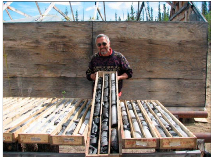
Figure 45. Coal seam in core from the Corduroy Mountain property near Division Mountain.
