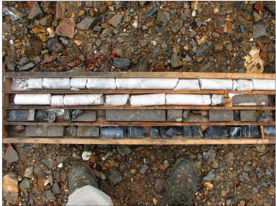
Figure 8. Massive pyrrhotite-pyrite mineralization in drill core from the Calcite zone, a new discovery at Ketza River.
