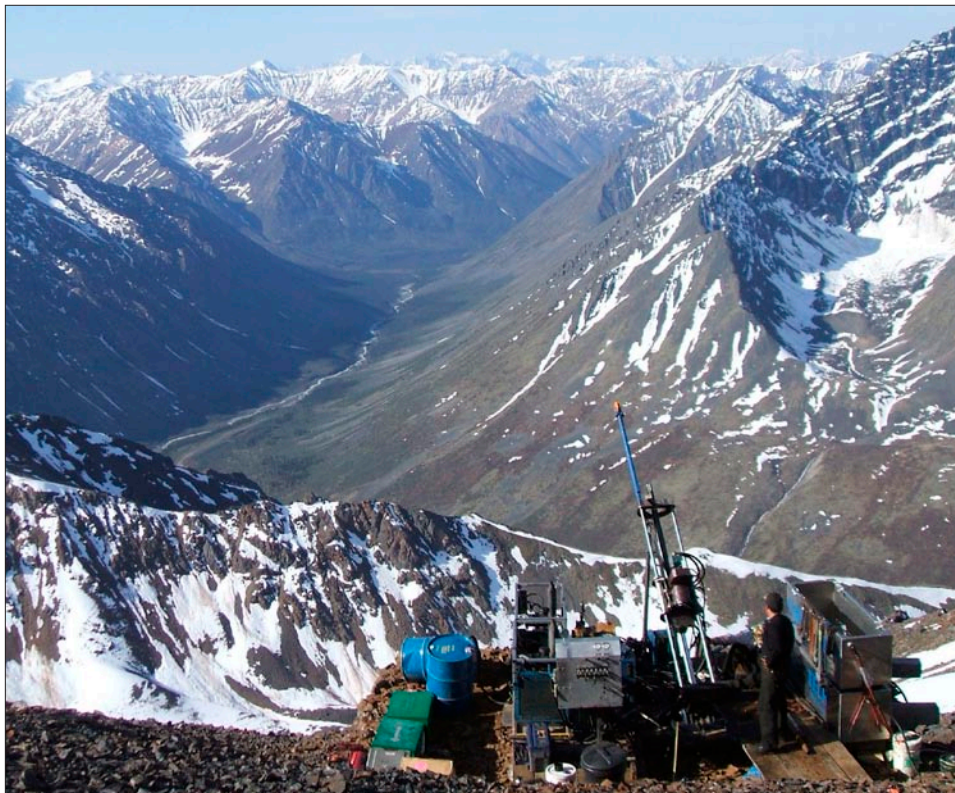
Figure 41. Helicopter supported, low-impact drillings on Lumina property.
