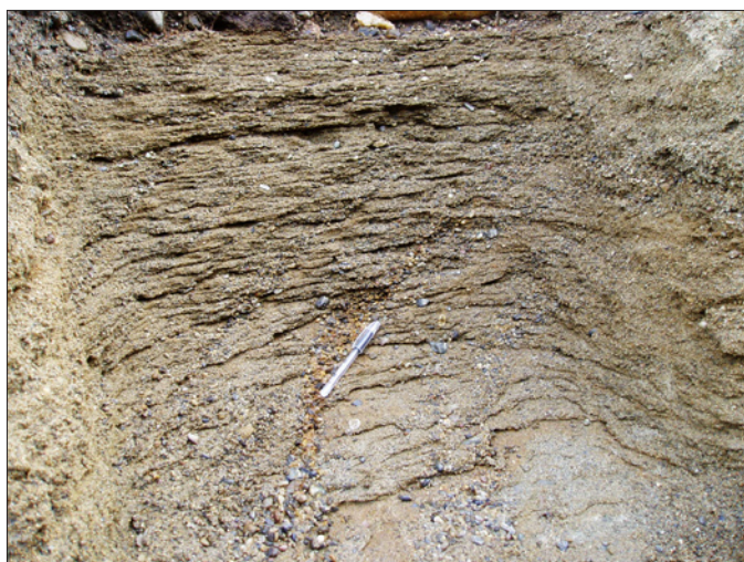
Figure 8. Weak cross-bedding at Diversion Creek; pen in photo is parallel to cross-bedding. This face was excavated in order to obtain a strike and dip of cross-bedding.
