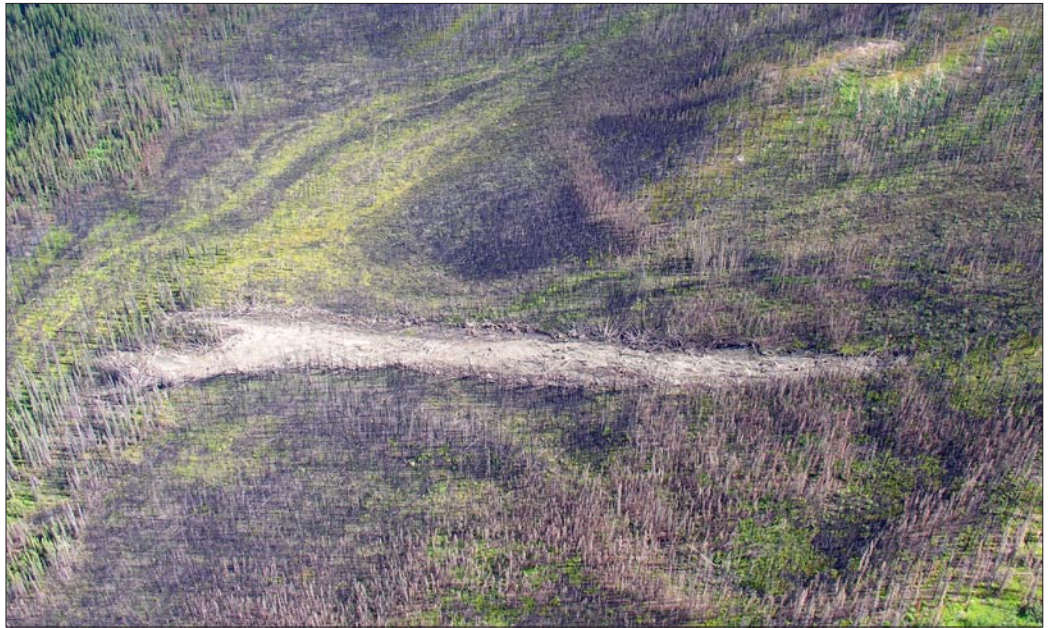
Figure 4. A large active-layer detachment was initiated on a gentle north-facing slope near the mouth of Excell Creek following forest fires in 2004. The failure is estimated to be approximately 300 m long. Photo taken in July, 2006.
