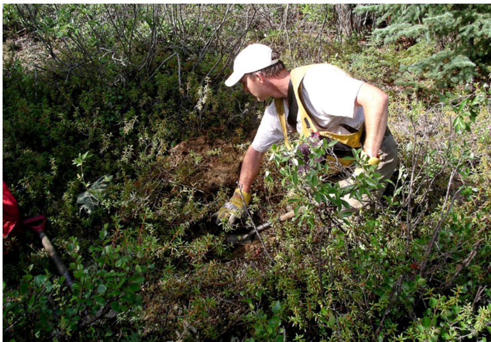
Figure 30. Geologist Jeff Bond (YGS) demonstrating how to conduct an MMI survey at King Lake copper property.
