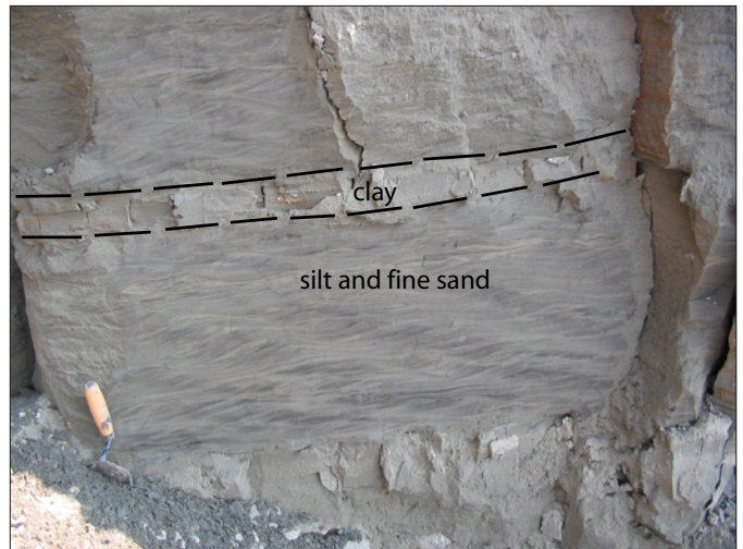
Figure 12. Stratified deltaic/lacustrine deposits within the lower reach. Massive clay alternating with ripple cross-laminated silt and fine sand.
