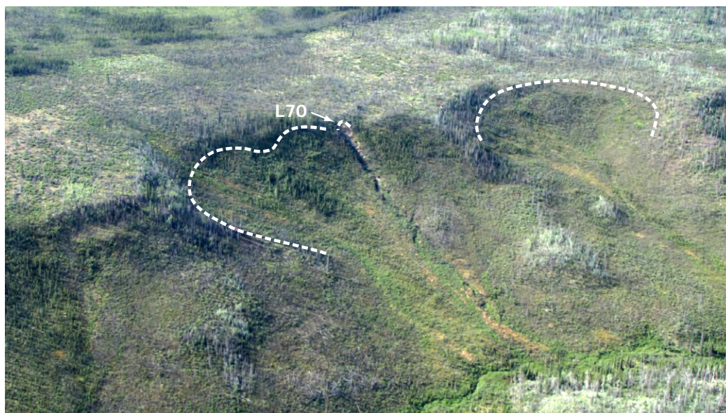
Figure 3. Retrogressive slump scars in Willow Hills (scalloped features cutting into upper bench); view is to the south. The upper bench is approximately 70 m above the valley bottom and consists of a glaciofluvial terrace underlain by ice-rich glaciolacustrine sediments. L70 represents a stratigraphic section location.
