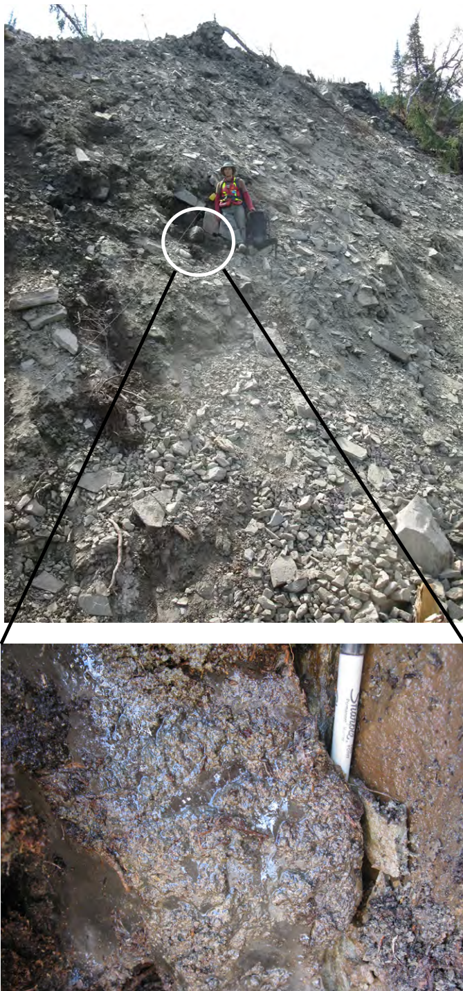
Figure 8. Ice lens observed at the front of a slumped block of highly broken-up schist.
