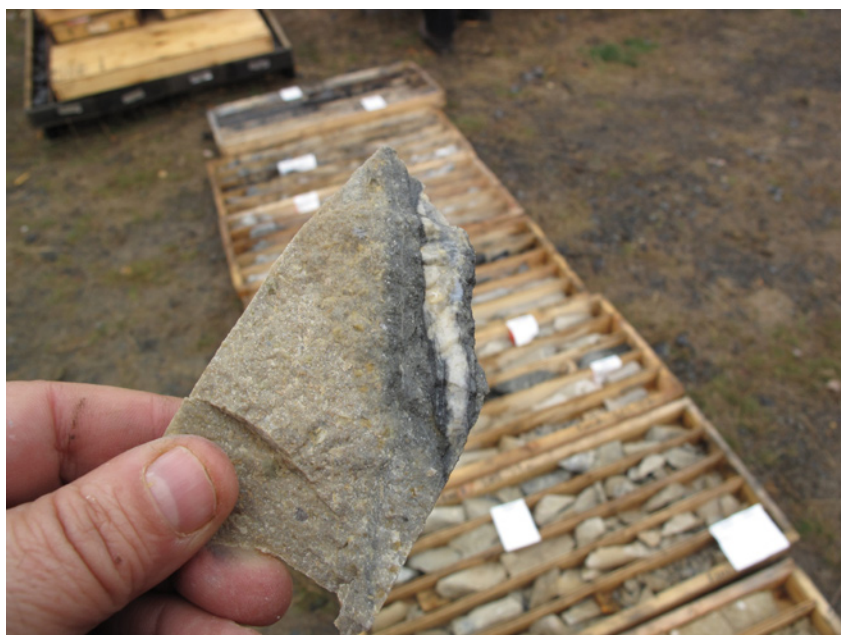
Figure 25. Altered quartz-monzonite dyke with cross-cutting stibnite vein from Brewery Creek property.
