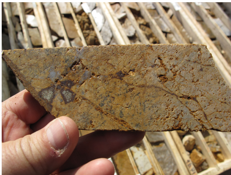
Figure 16. Disseminated pyrite mineralization in felsic rock at the White Gold property.
