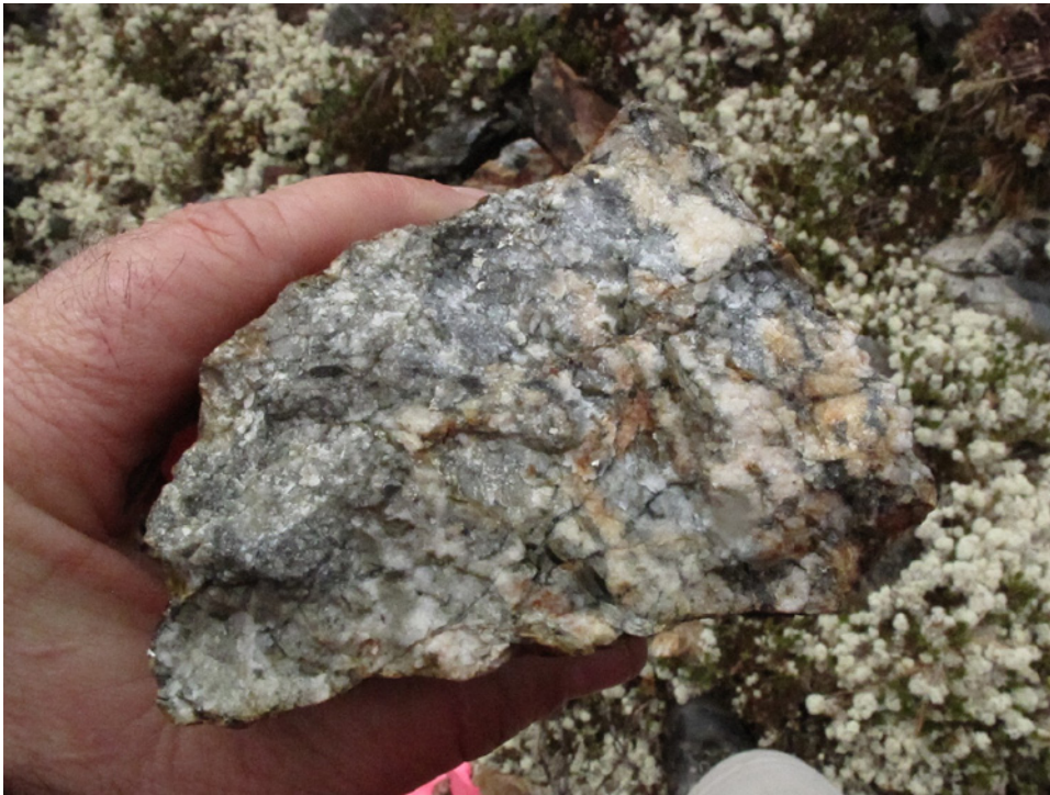
Figure 28. Quartz arsenopyrite vein from the Golden Culvert property.
