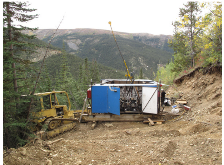
Figure 13. Diamond drill rig at the Tom zone on the Gold Dome property.
