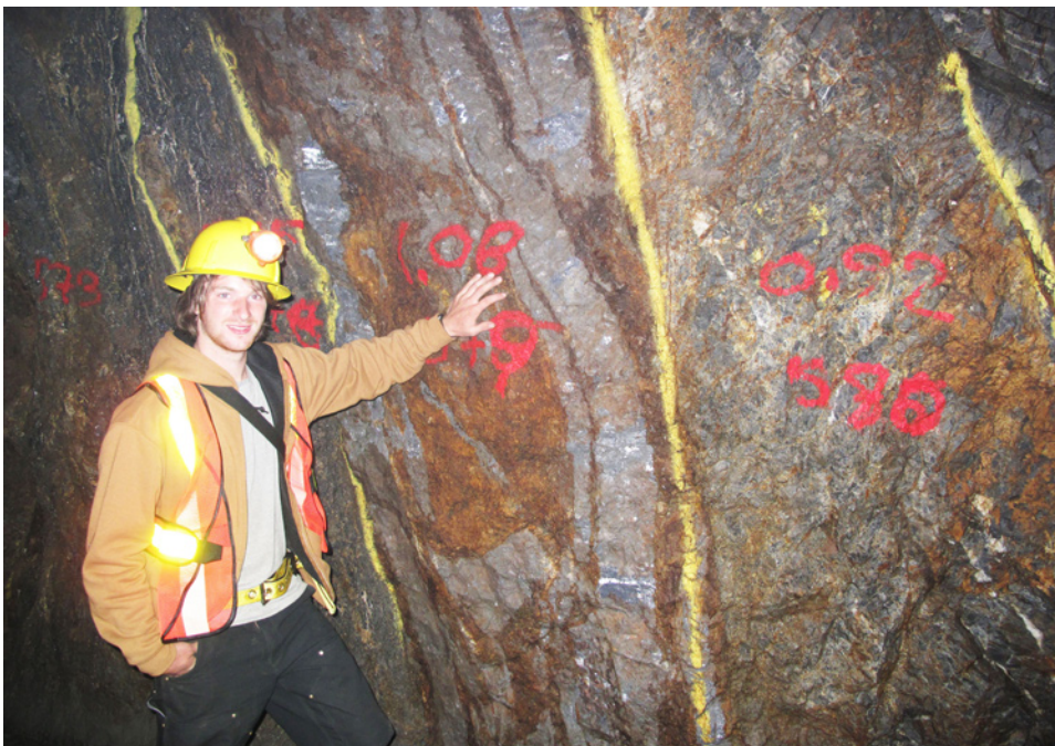
Figure 10. N. Goeppel, student geologist, underground at the Bellekeno deposit with high-grade galena-sphalerite-siderite vein.
