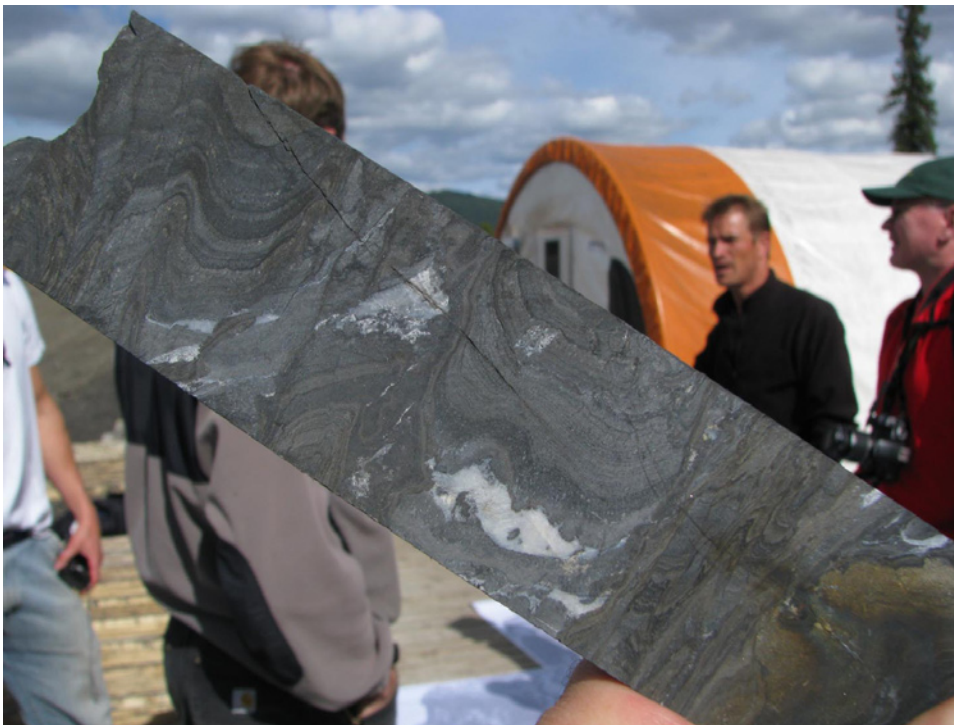
Figure 35. High-grade, deformed, laminated sphalerite-galena mineralization from the Selwyn SEDEX project.
