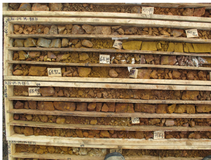
Figure 11. High-grade drillcore (Rau09-19) from the Rau property oxide zone.
