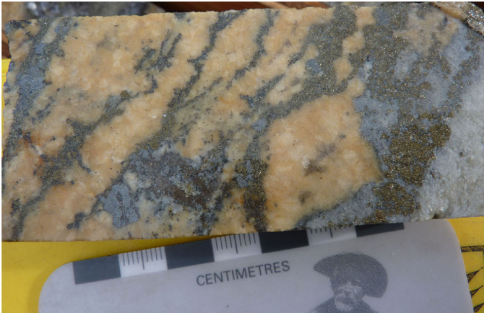
Figure 12. Sulphide replacement of dolomite from the Rau property.
