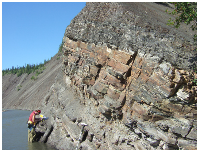
Figure 15. Outcrop of black, organic-rich shale interval, approximately 200 m above the base of the Imperial Formation on Tetlit Creek. This interval is 165 cm thick.
