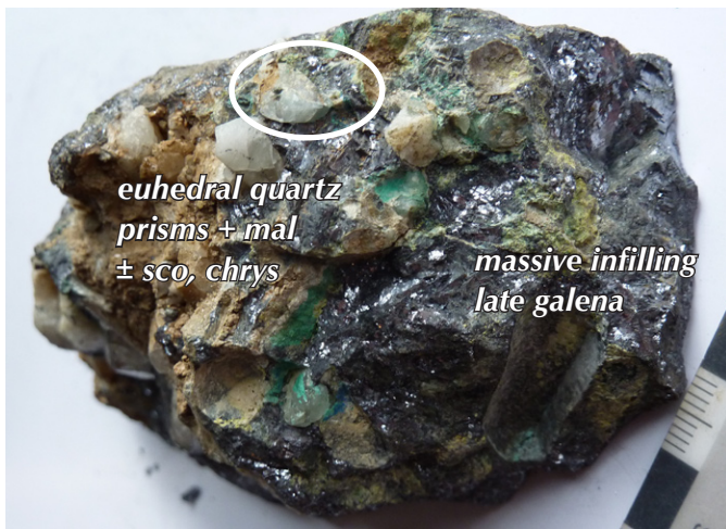
Figure 14. Euhedral quartz prisms with cubic galena inclusions surrounded in banded base-metal mineralization (galena + malachite \pm scorodite, chrysocolla). mal = malachite, sco = scorodite, chrys = chrysocolla.
