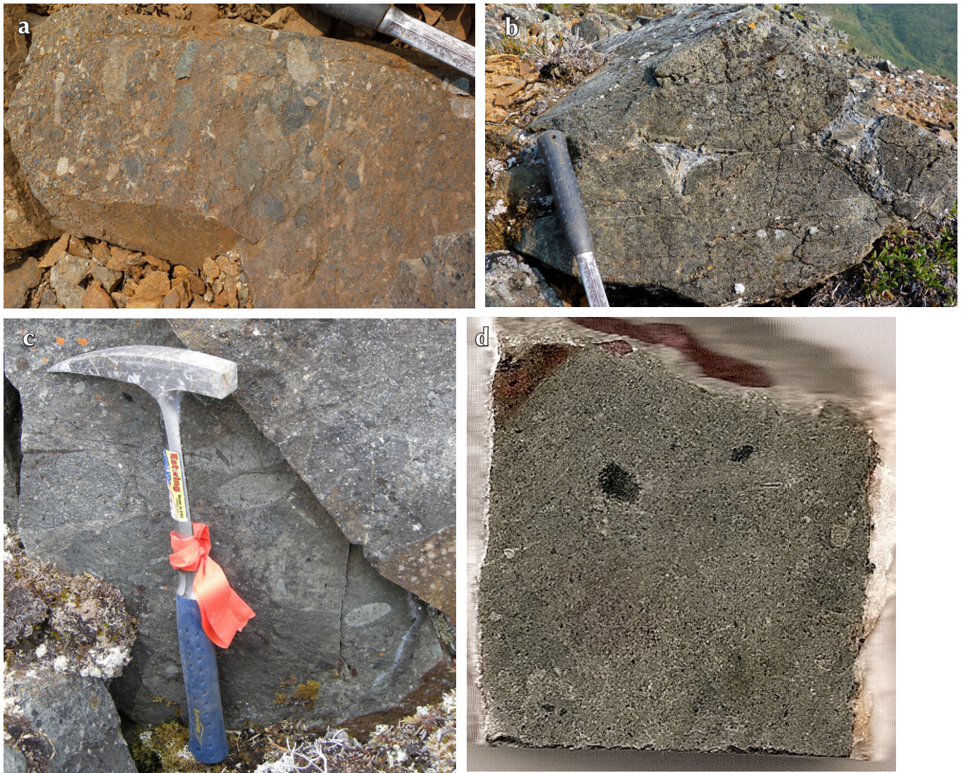
Figure 5. McKay Hill country rocks: (a) conglomerate, (b) pillow basalt, (c) volcanic tuff, and (d) andesite (locally hornblende-phyric).
