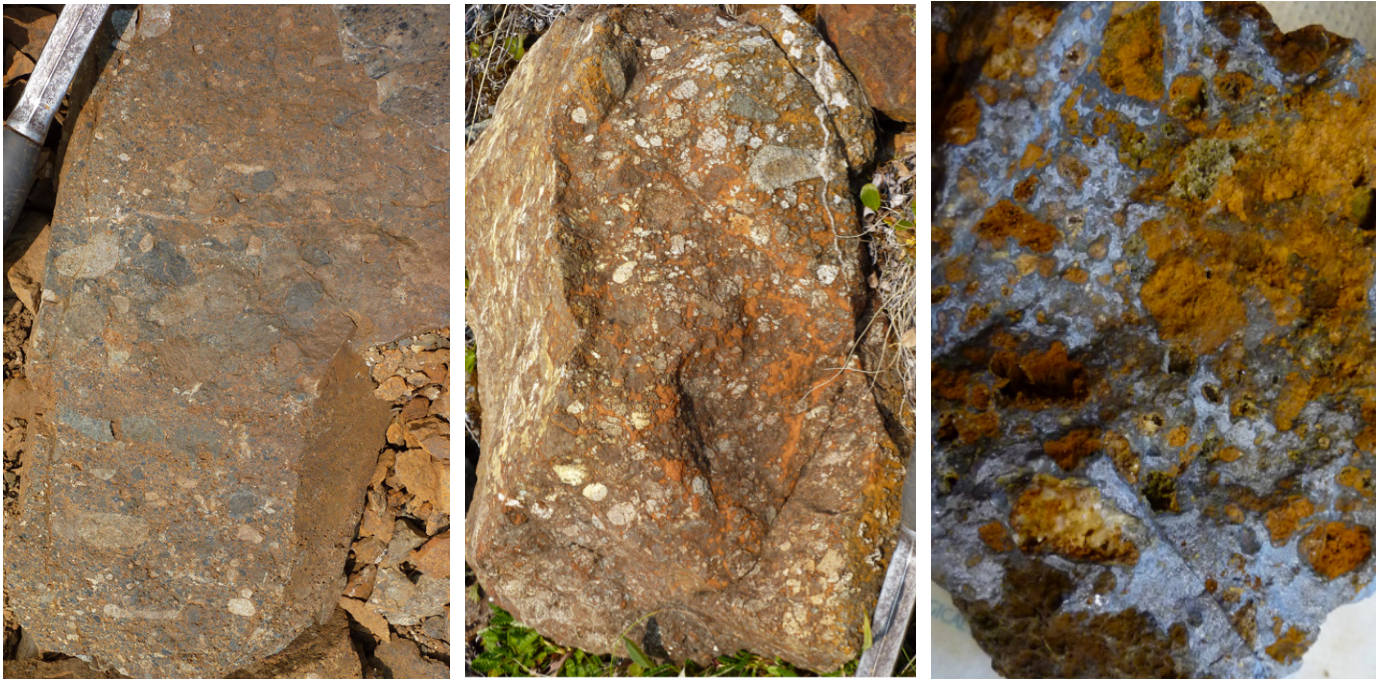
Figure 13. Progressive Fe-carbonate alteration and destruction of the conglomerate framework clasts with late-stage matrix replacement of galena.
