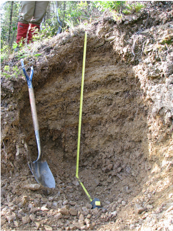
Figure 4. Weathered bedrock colluvium which typically mantles valley sides and uplands. Note angular coarse fragments and stratification resulting from prolonged modification by periglacial processes and mass movement. Loess is commonly incorporated into the near-surface horizons.
