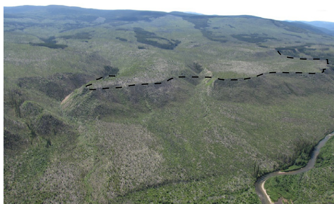
Figure 8. Glaciofluvial delta formed at the outlet of a small meltwater channel in a west-flowing tributary to the Beaver River (Fig. 3). These deposits often consist of well-sorted sand, and mixed sand and gravel. Dashed black line marks the front edge of the delta surface.
