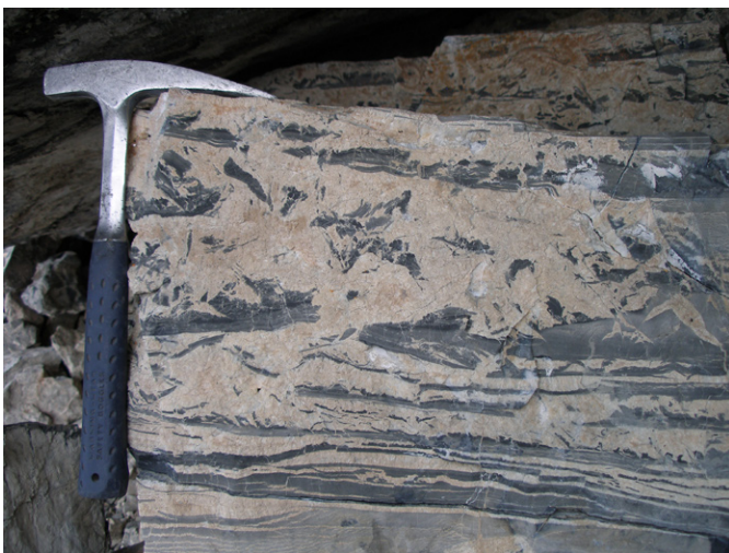
Figure 10. Pervasive, late brecciation in thin-bedded dolostone; breccia interstices are filled with coarsely crystalline dolospar.
