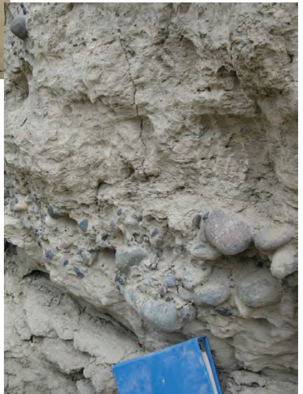
Figure 18. Gap-graded, polymictic, well rounded coarse gravel (including cobbles), in a matrix of silt and clay, at station MAB 09-20-02.
