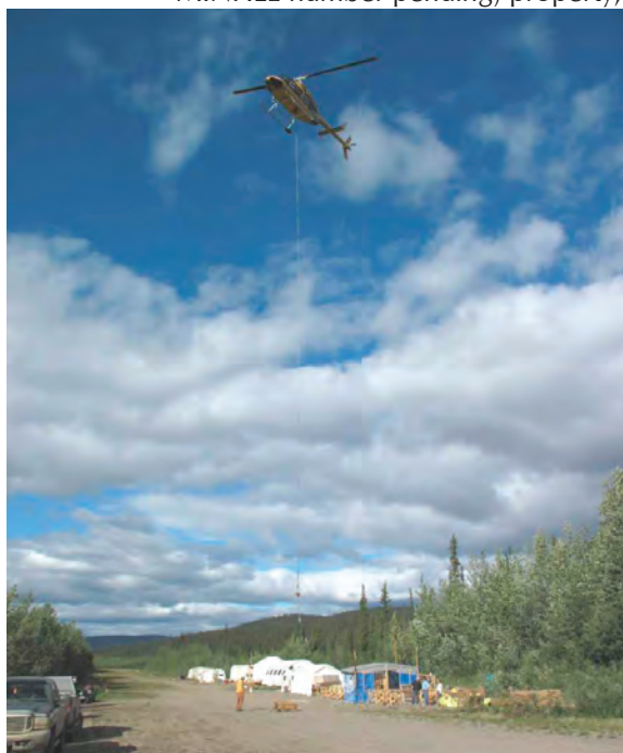
Figure 15. Slinging core boxes at Aldrin Resources' Keystone property.
