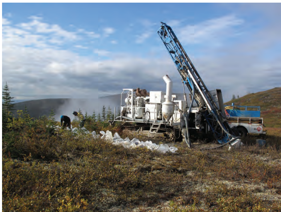
Figure 25. Reverse circulation drilling on Gold Dome.
