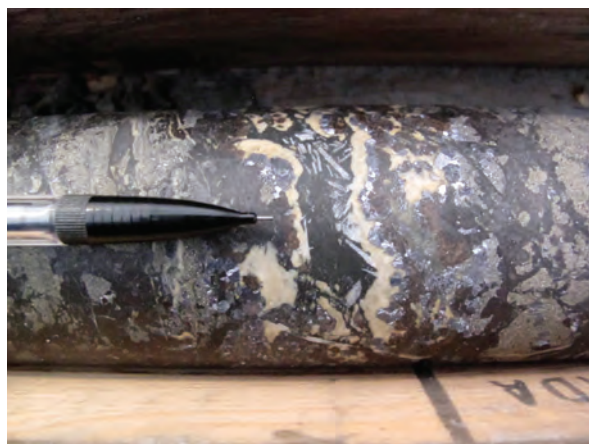
Figure 21. Pyrite-sphalerite-galena-carbonate vein in drill core from the Klaza gold-silver property.
