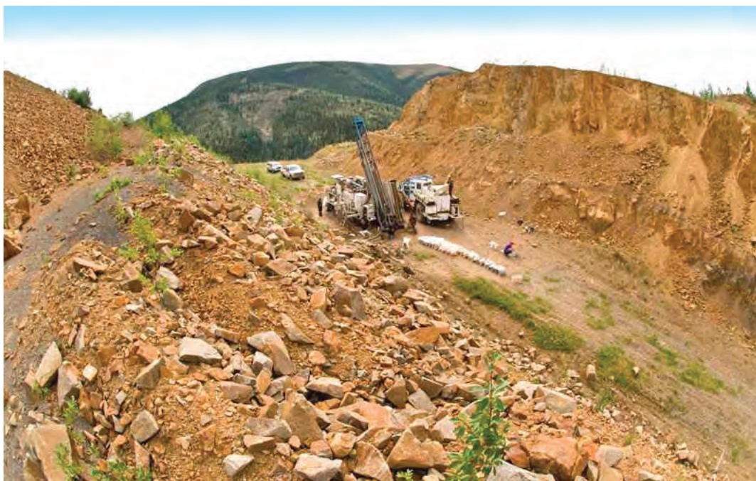
Figure 27. Reverse circulation drill at Brewery Creek gold property. Photo by Cathie Archbould from www.goldenpredator.com .
